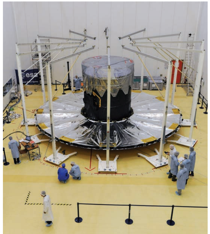
Gaia is fitted with a ten-metre diameter Sunshield Credit: ESA
