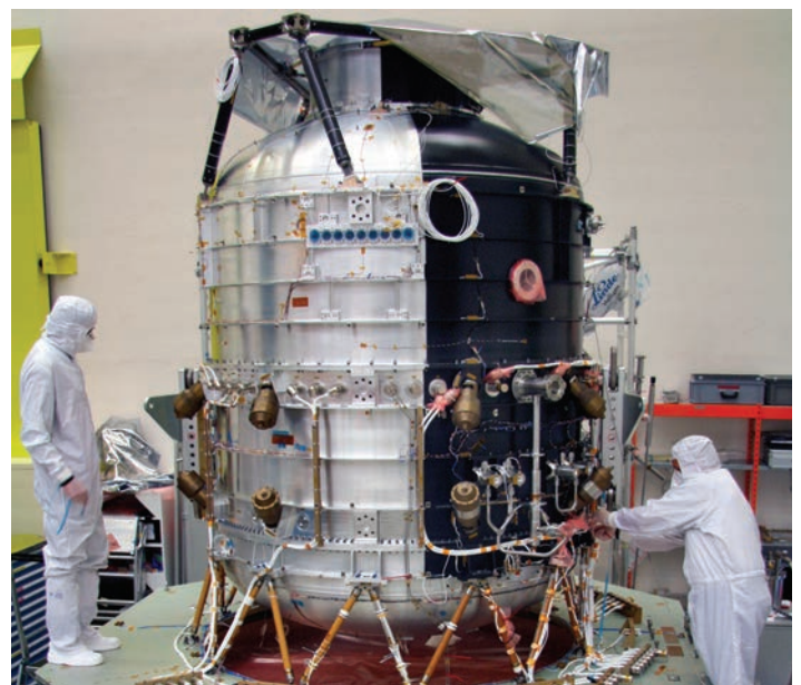
Herschel's cryostat vacuum flask was filled with 2000 litres of liquid Helium Credit: ESA
