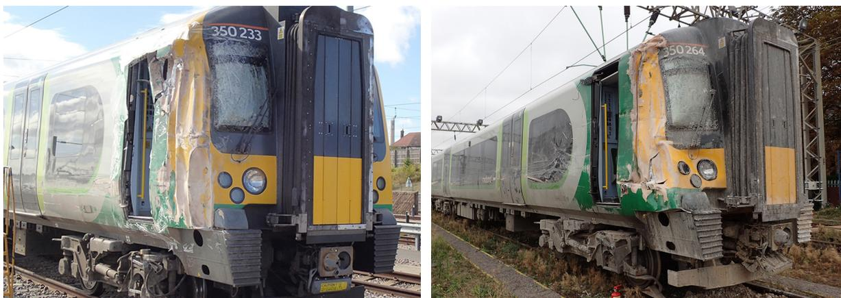
Figure 17a and b: Front view of train 2Y59 (unit 350233) and train 2K04 (unit 350264) following recovery from the tunnel
