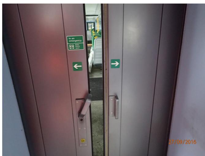
Figure 18: Maximum width that the sliding cab-saloon doors could be opened following the accident
