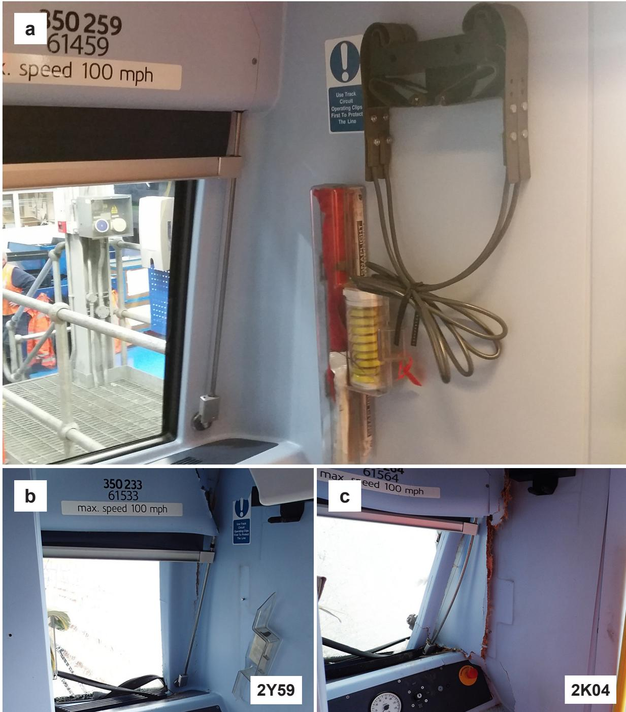
Figure 19a, b and c: Photographs showing the location of cab emergency equipment in an unaffected train, and damage to the leading cabs of trains 2Y59 and 2K04
