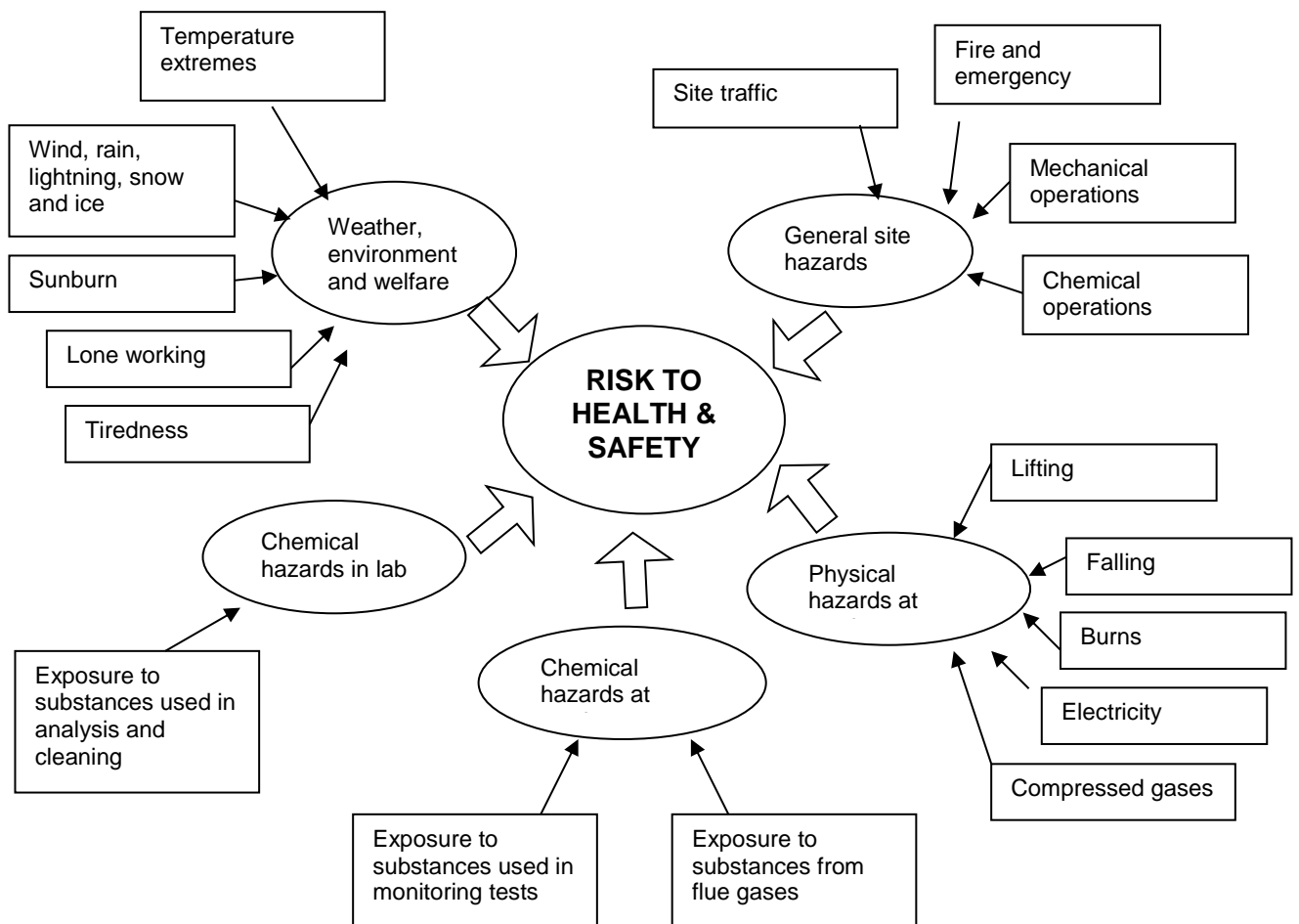
Figure 9.1 Most prominent hazards associated with stack monitoring
