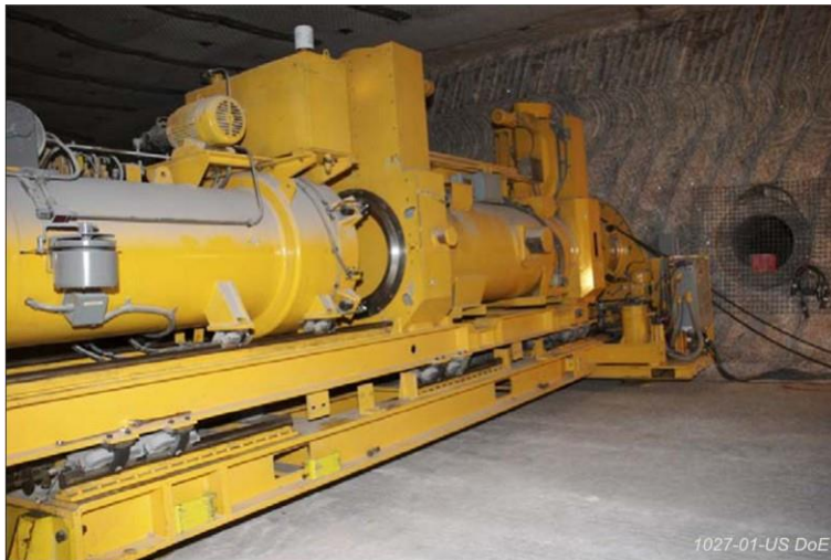
Figure 34 Test emplacement of a remote-handled TRU waste container into a horizontal borehole in the wall of a disposal room.
