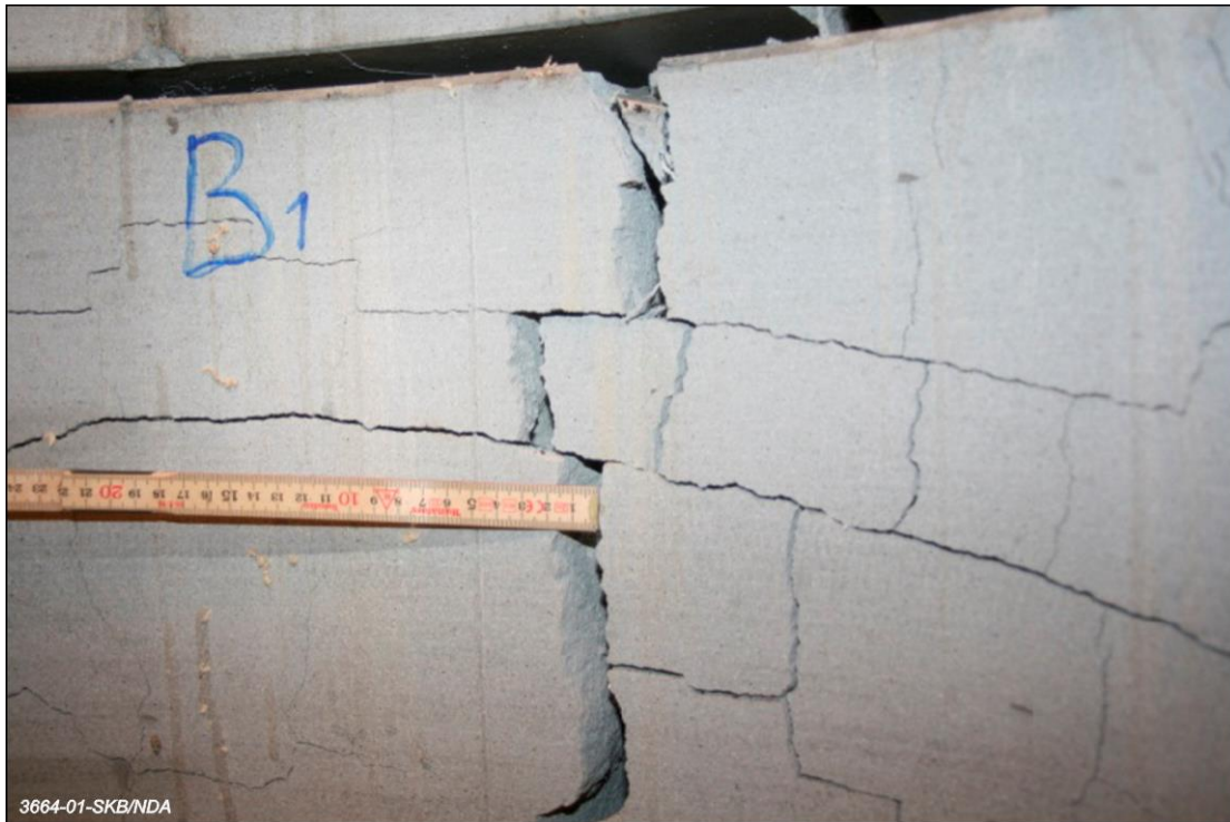
Figure 6 Cracks observed from the inside of ring-shaped bentonite blocks (from a full scale test carried out by SKB [57]).
