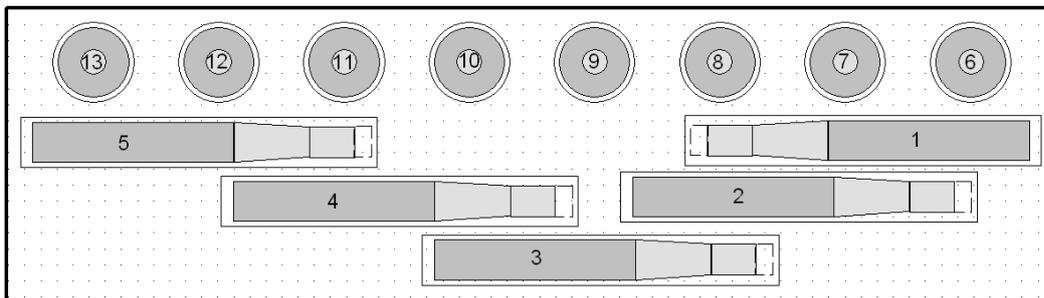
**Figure 1: Synergy 2 detector layout: 1 – 5 NaI detectors, 6 – 13 FIDLER detectors.**
