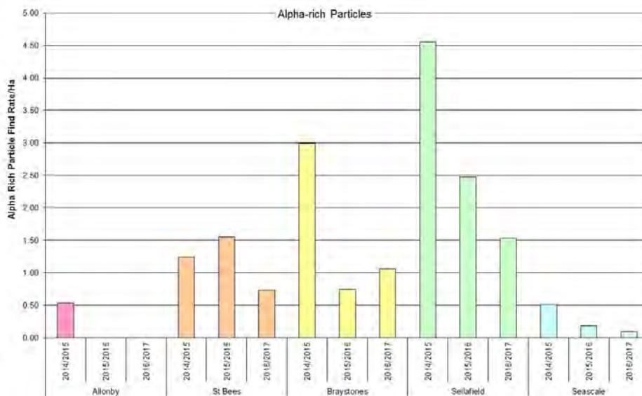
**Figure 10: Alpha rich particle find rates since the introduction of Synergy 2.**
