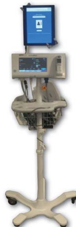
Figure 1 New devices with a barcode scanner and a Wi-Fi enabled touchscreen tablet
