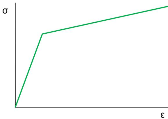
**Figure 13: Linear elastic-plastic material model with strain hardening**
