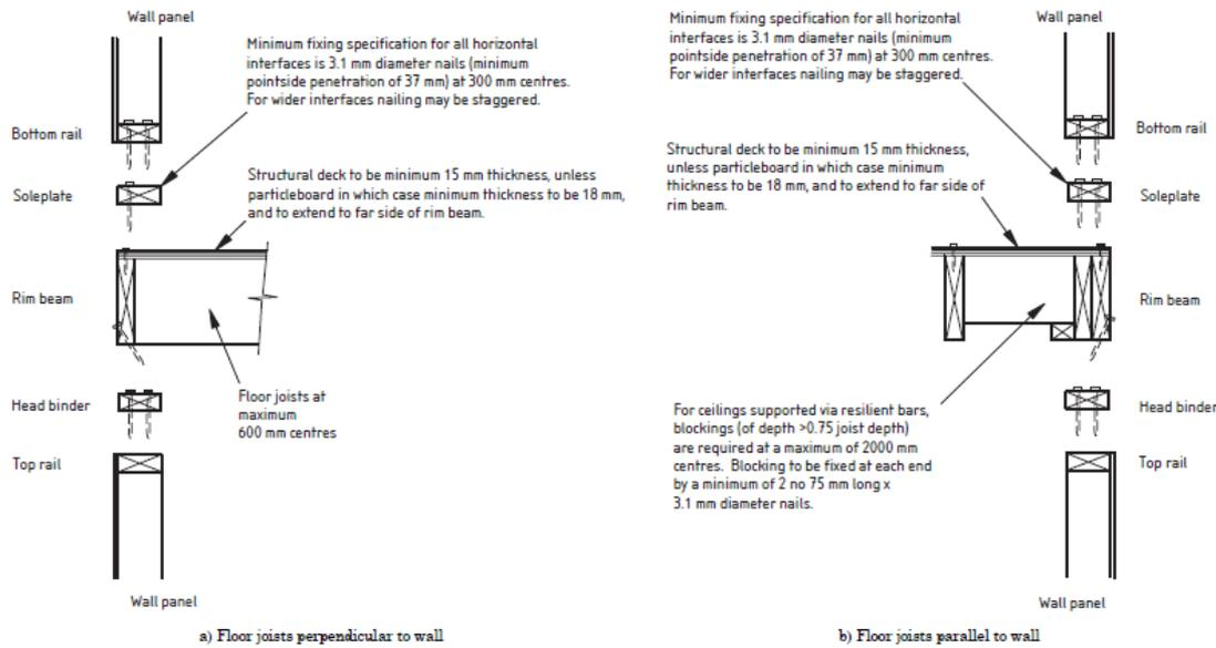
Figure M.3 — Floor deck — wall panels intersection: Exploded view
