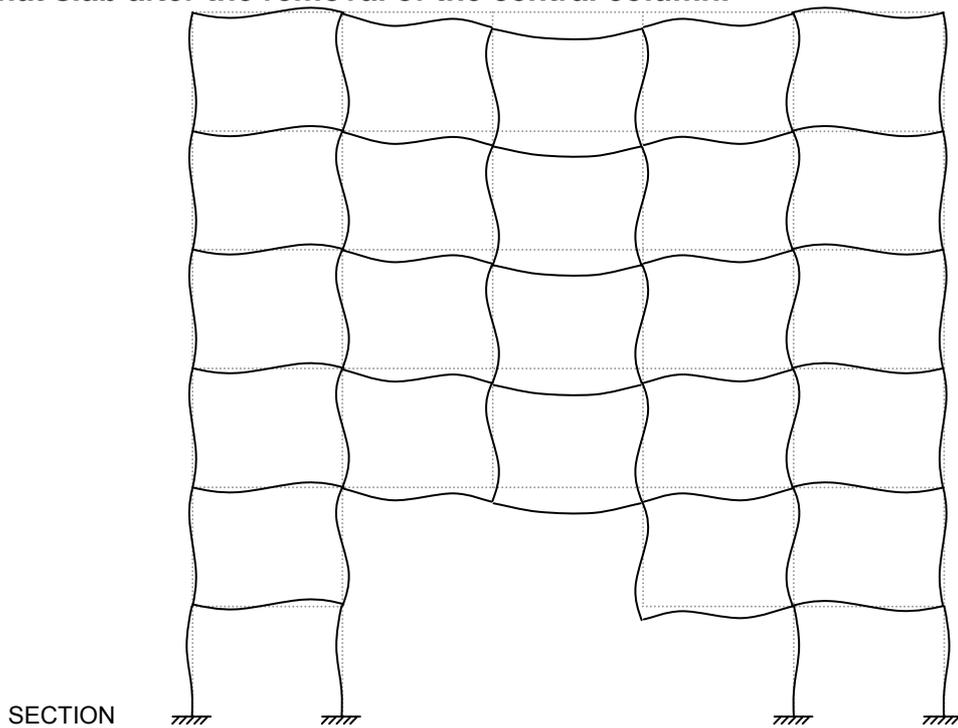
**d: Mechanisms to resist collapse. Vierendeel action due to moment capacity in beam/column connections following loss of two columns (of which one is lost over two storeys) and the first floor beam over two structural bays.**
