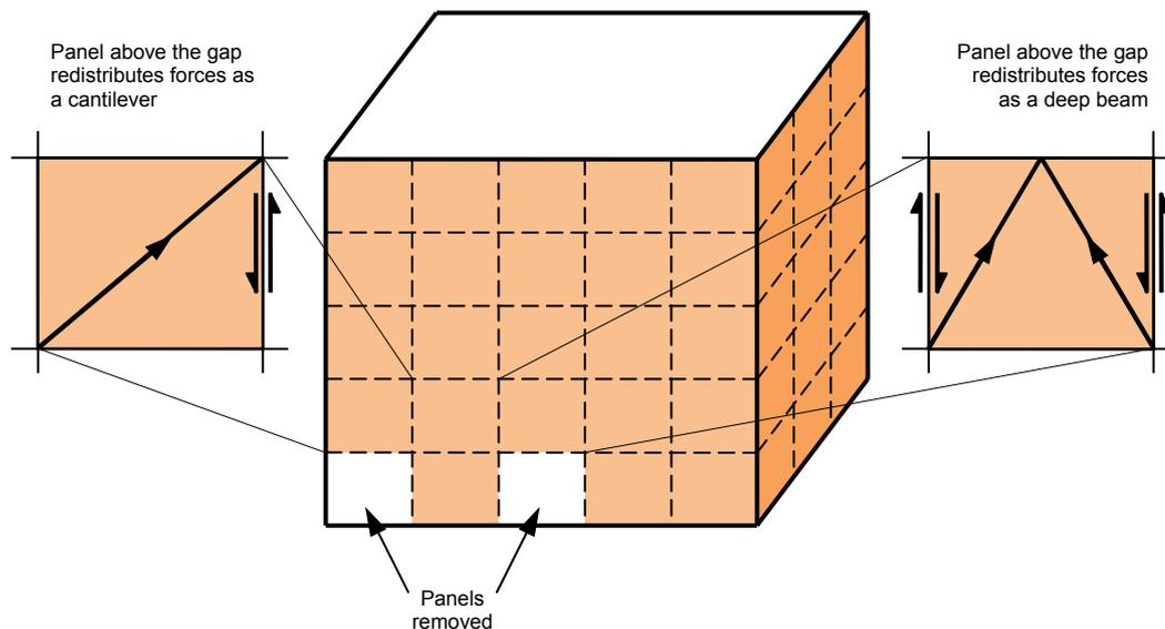
**Figure 21: Spanning of standard 2.4m x 4.2m long platform timber frame wall panels Adapted from Grantham (2003). © Arup**
