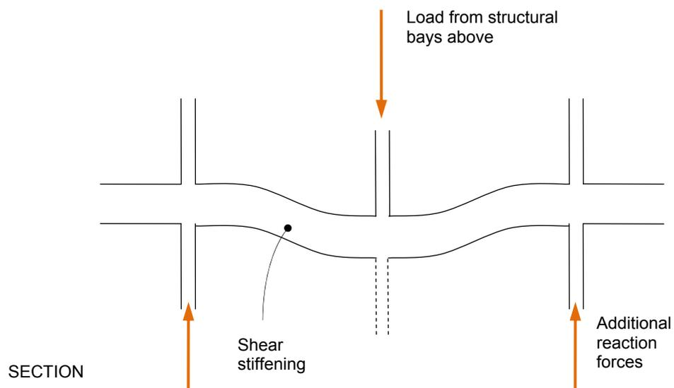
**b: Mechanisms to resist collapse. Shear deformation of deep transfer/spandrel beams.**
