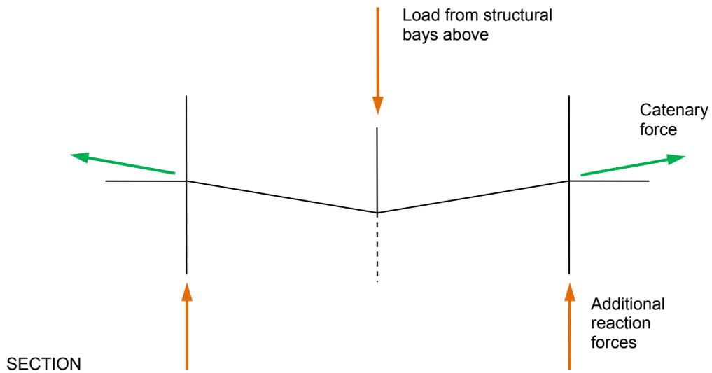
**Figure 10: Mechanisms to resist collapse**
