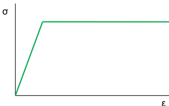
**Figure 12: Linear elastic-perfectly plastic material model**
