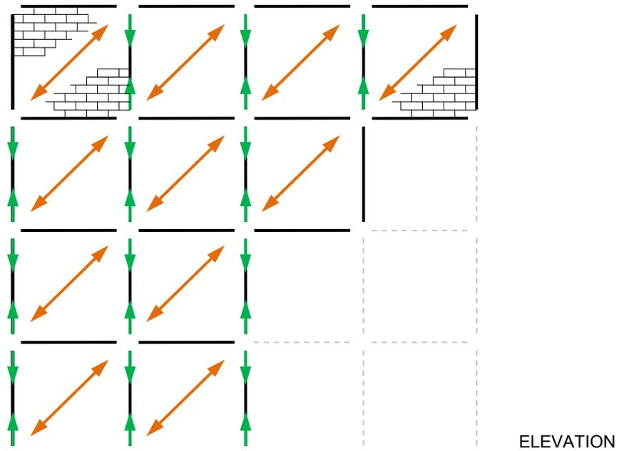
**f: Mechanisms to resist collapse. Compressive strut action in masonry panels**
