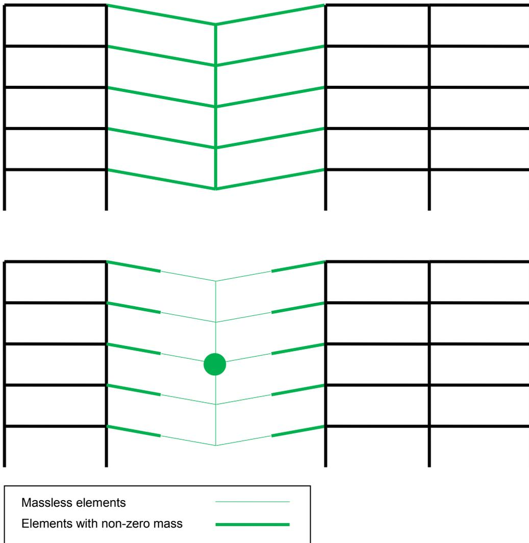
**Figure 14: Idealisation of structural bay as a single degree of freedom**
