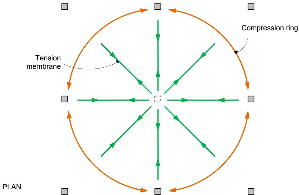
**c: Mechanisms to resist collapse. Tensile membrane developed in a flat slab after the removal of the central column.**
