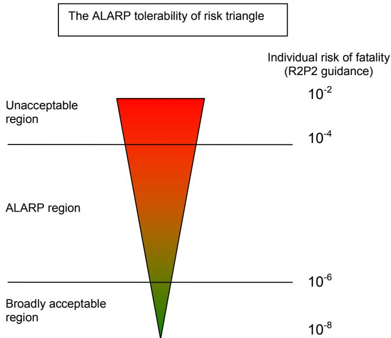
**Figure 1: The ALARP tolerability of risk triangle**
