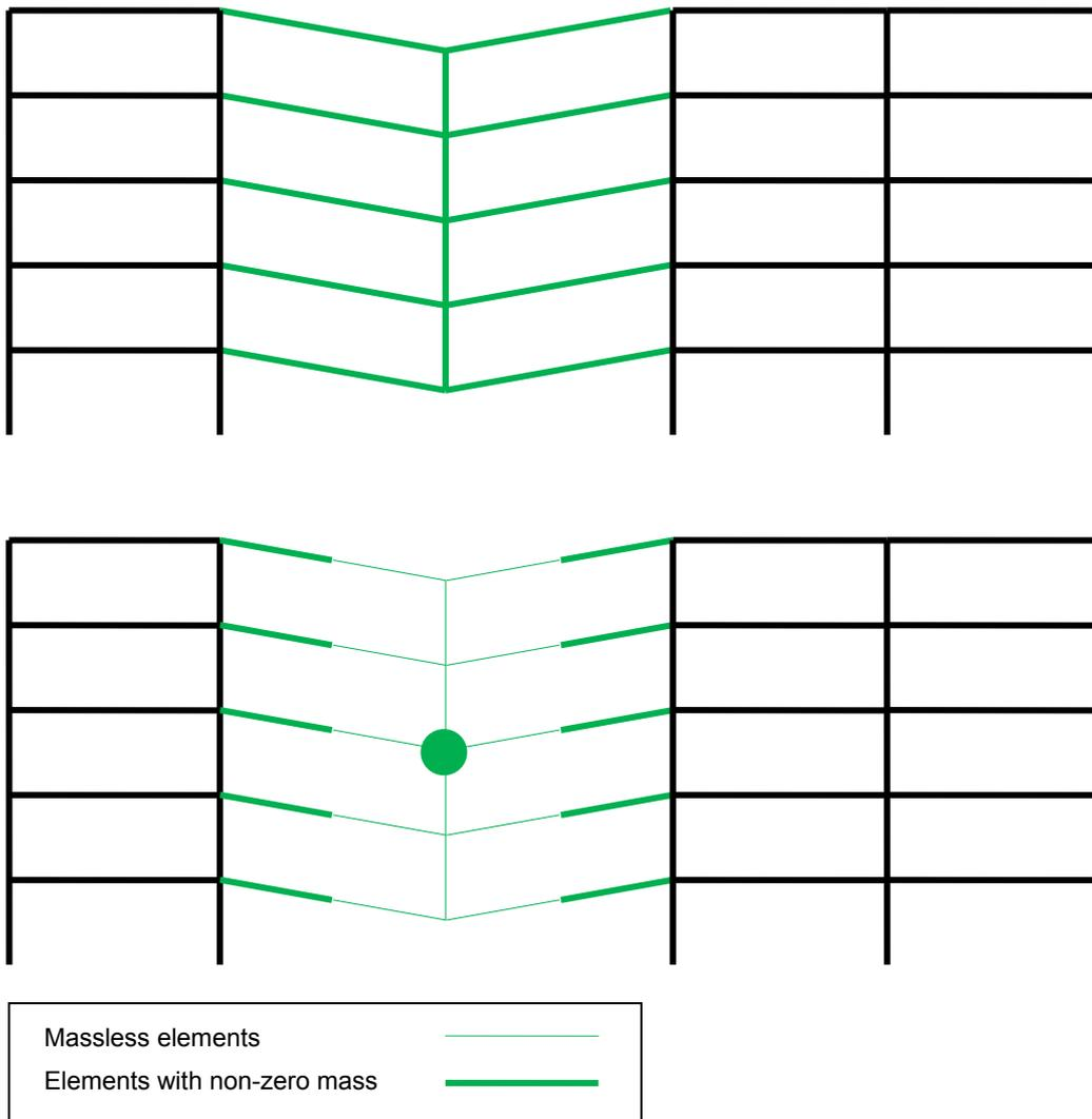
**Figure 14: Idealisation of structural bay as a single degree of freedom**
