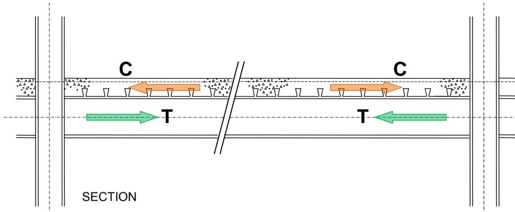
**e: Mechanisms to resist collapse. Compressive arching action between composite metaldeck slab and steel floor beams.**
