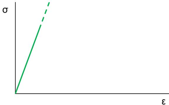
**Figure 11: Linear elastic material model**
