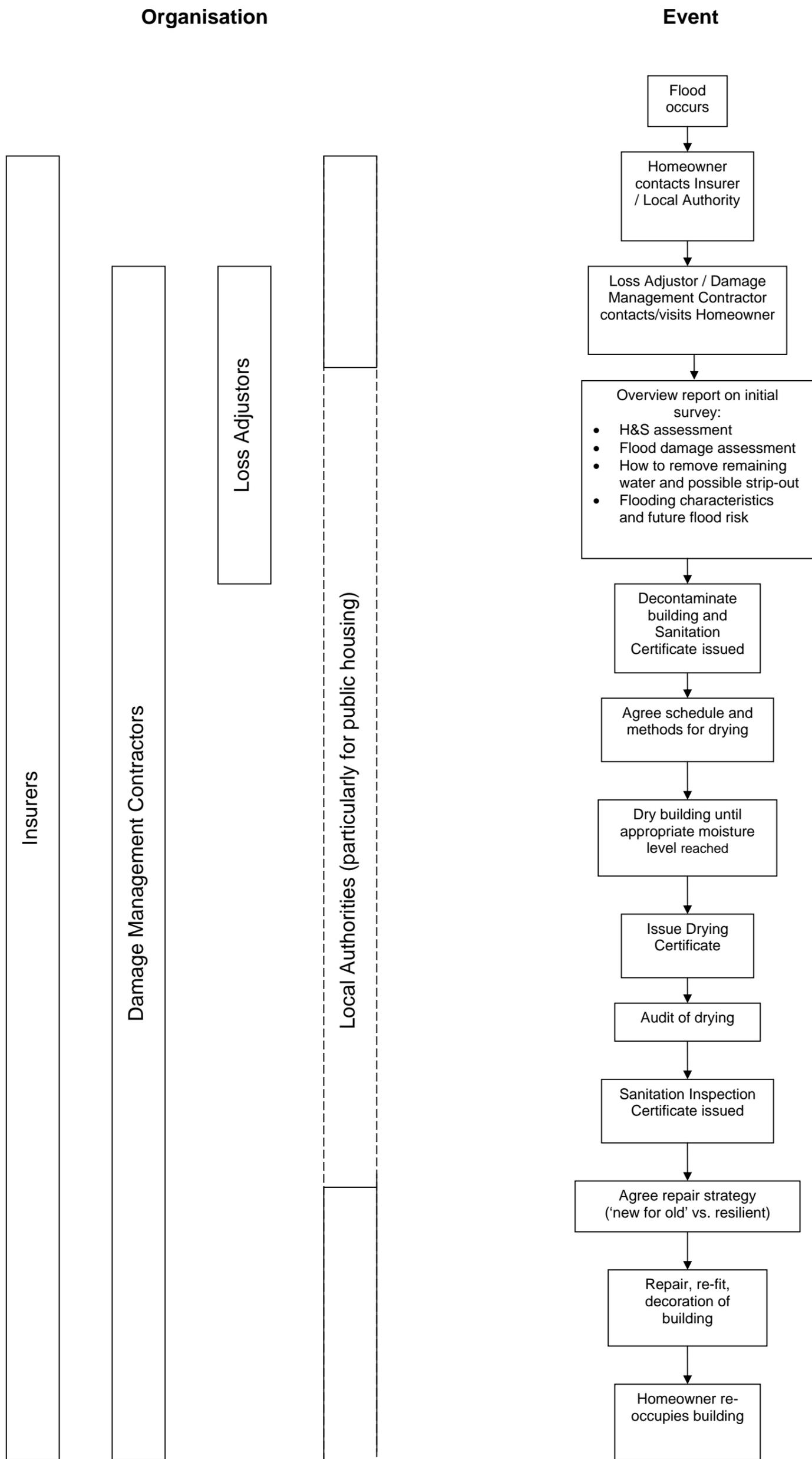
Figure 1.1 Stages in restoration of flooded buildings
