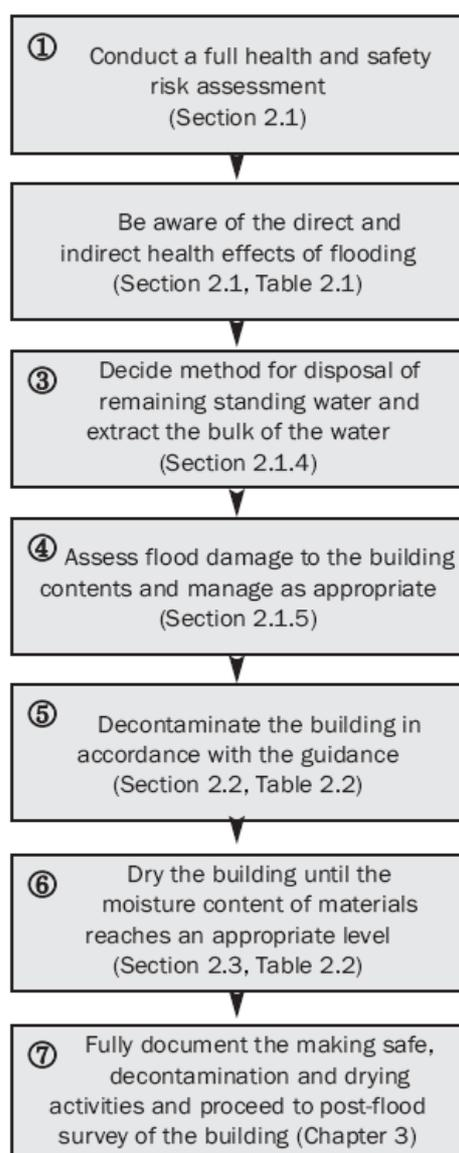
**Figure 2.1** Method for safe and effective decontamination and drying of a flooded building
