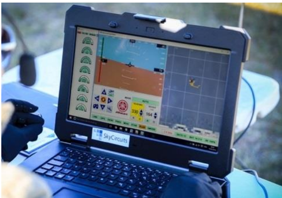
Managing and monitoring drone operations using a SkyCircuits Ground Control Station. Image copyright: SkyCircuits
