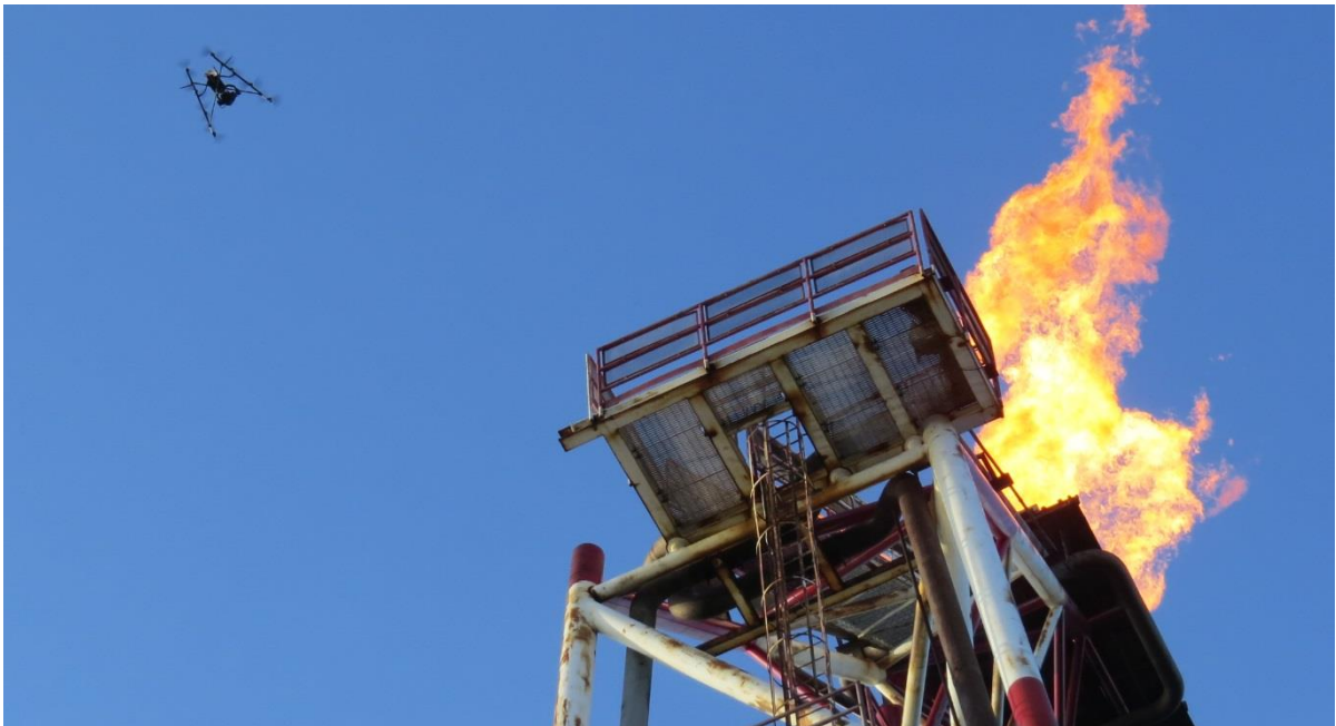
A drone being used to inspect an oil rig gas flare. Image copyright: Sky-Futures
