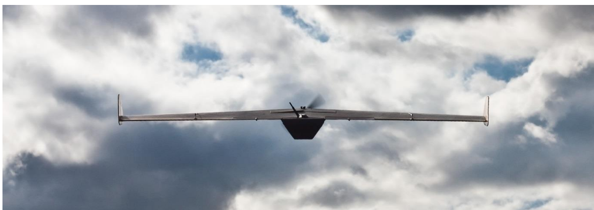
Callen-Lenz lightweight drone used in infrastructure survey. Image copyright: Callen-Lenz
