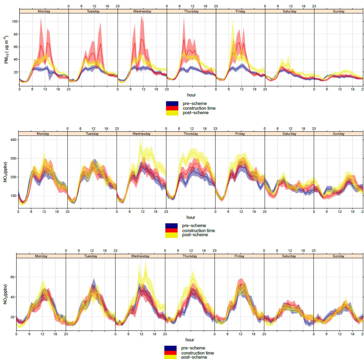
Figure 19. Mean hourly increments above background of PM<sub>10</sub>, NO<sub>x</sub> and NO<sub>2</sub> measured at Marylebone Road for each day of the week for the pre-scheme, construction and post-scheme periods.
