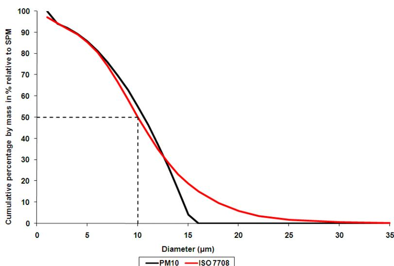
Figure 2: Cumulative percentage by mass of the PM<sub>10</sub> fraction and the thoracic fraction (ISO 7708) relative to Suspended Particulate Matter (CEN, 1998)
