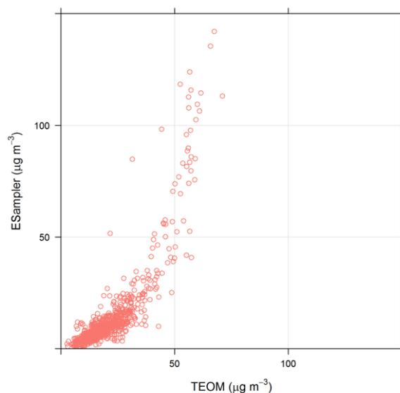
Figure 18: Scatterplot showing relationship between the TEOMvcm at Richmond Barnes and the mean of the two ESamplers at Garth Road, Merton
