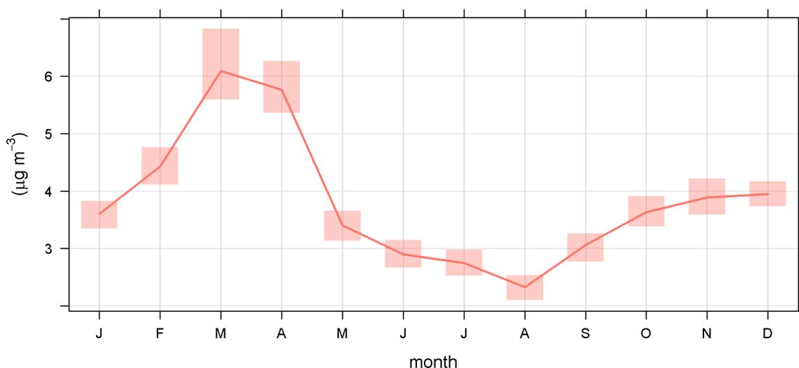
Figure 1: Volatile PM concentrations measured using the FDMS at North Kensington
