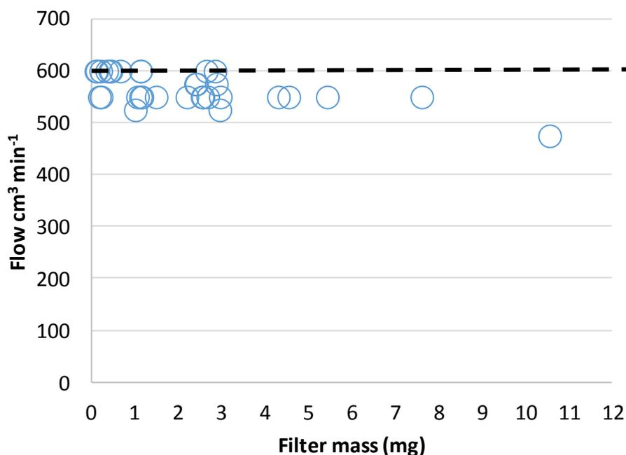
Figure 4 Flow measurements and filter mass for four examples of instrument type I. Flow was measured without intervention from the filter change. The dotted line represents the target flow of  $600 \text{ cm}^3 \text{ min}^{-1}$
