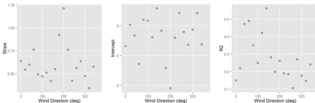
Figure 14: Correlation between the Osiris and FDMS  $PM_{10}$  grouped by 10 degree wind sector
