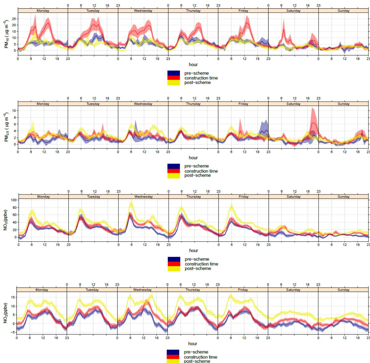
Figure 20. Mean hourly increments above background of PM<sub>10</sub>, PM<sub>2.5</sub>, NO<sub>x</sub> and NO<sub>2</sub> measured at Bexley 7 for each day of the week for the pre-scheme, construction and post-scheme periods.
