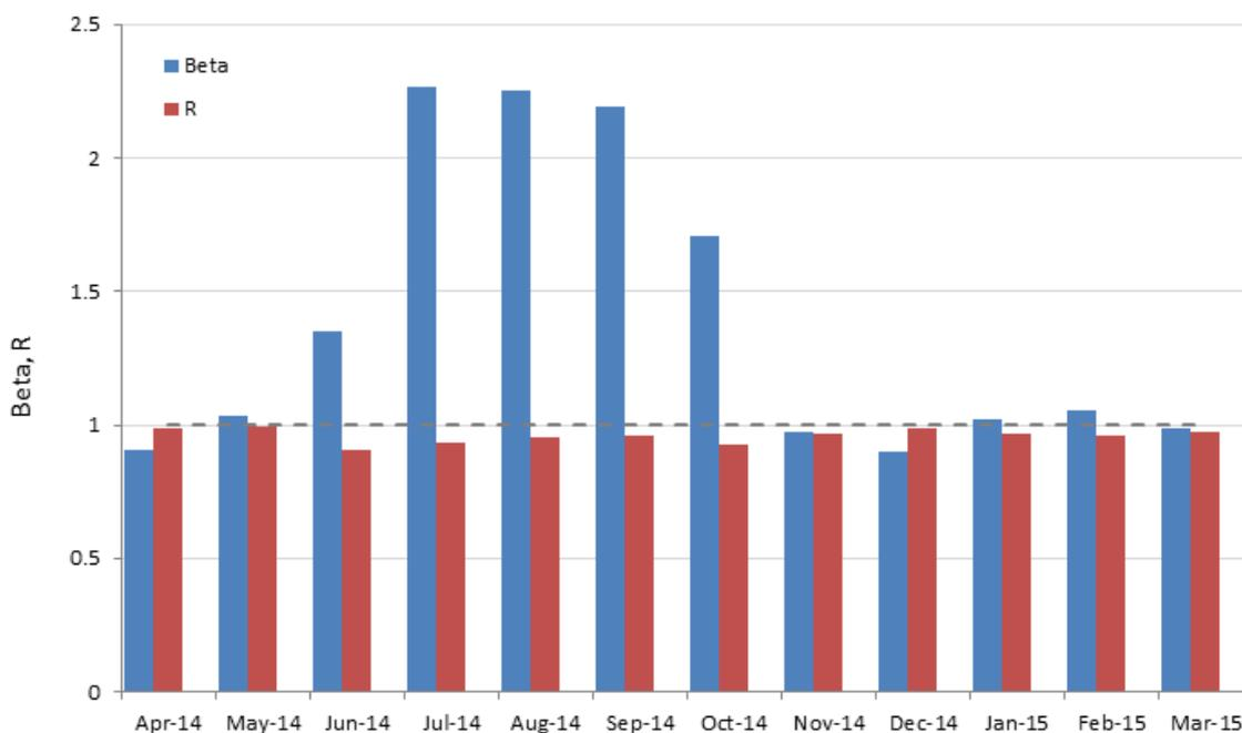
Figure 13 Monthly RMA regressions for instruments H and I. Regression gradient beta and correlation R are shown. Regressions were undertaken for hours 1-3 each night.
