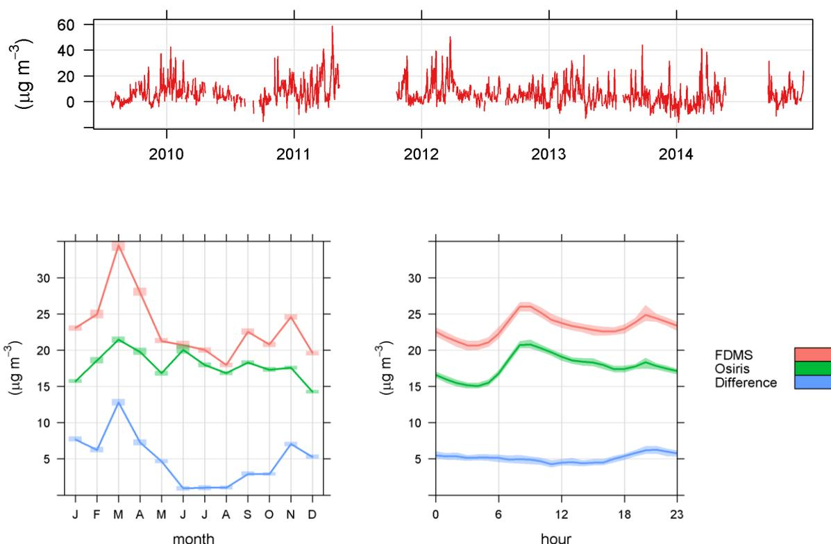
Figure 7: Measurements from the FDMS and Osiris at Coopers lane. The top panel shows the daily mean difference between the instruments. The lower panels show the difference along with the mean measurements from each instrument. This is shown as a monthly mean (left) and as a diurnal mean (right).
