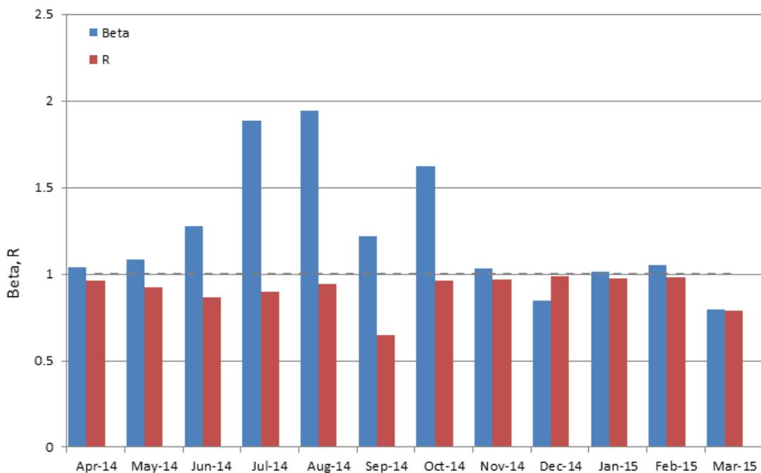
Figure 14 Monthly RMA regressions for instruments H and I. Regression gradient beta and correlation R are shown. Regressions were undertaken from Sundays.
