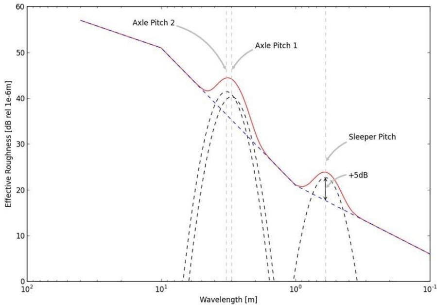
2.1.13 In Figure 2, the combined roughness of wheels and rails is denoted by the light blue checked line. Parametric excitation from axles is denoted by the dark blue checked line. The effective roughness term used in the speed correction is denoted by the red line.
