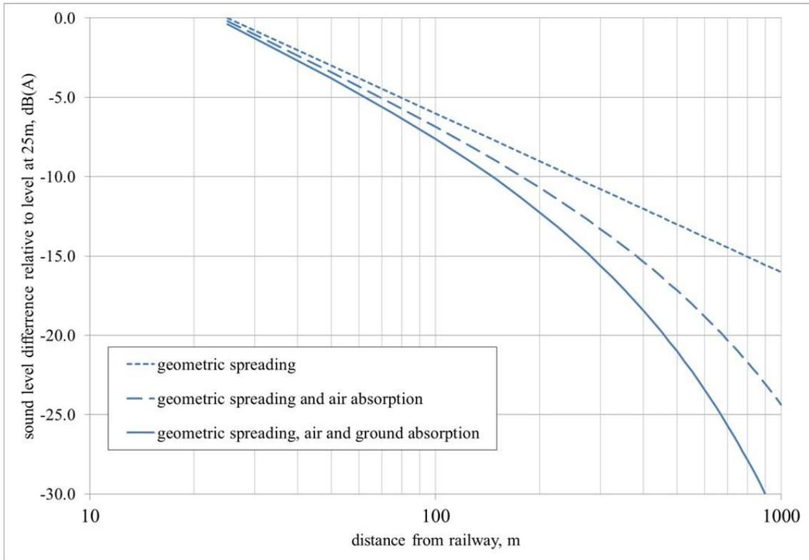
Figure 15: Effect of ground and air absorption on sound level (300m)
