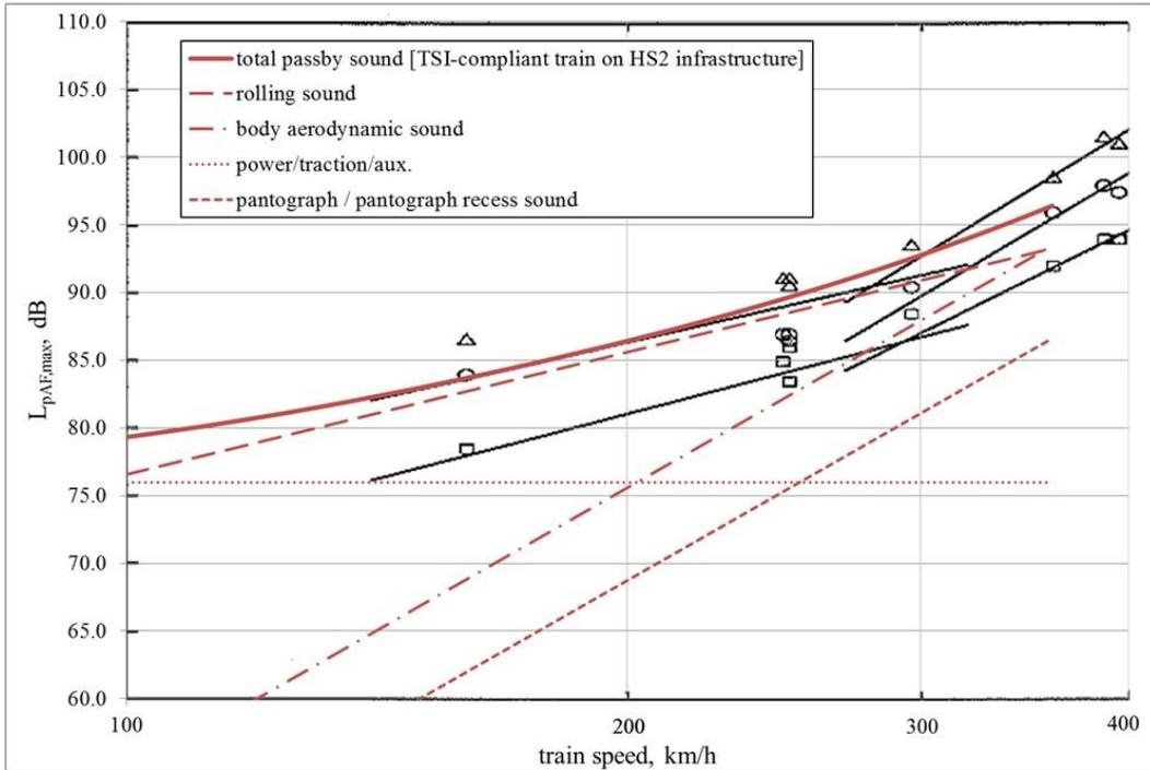
Figure 4:  $L_{pAeq,tp}$  vs speed for total and source component pass-by sound at 25m from the track predicted using the HS2 trains source terms.
