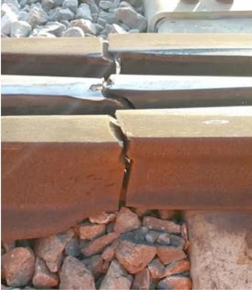
The picture on the left is a cracked crossing at Balham on 5<sup>th</sup> December, 2016 which caused significant delay. The cause is not known at the time of writing; it could have been related to drainage, sleepers, ballast or metallurgical causes.
