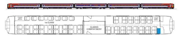
Figure 3: Layout of the Class 442 unit and detail of middle carriage (courtesy of GTR)
