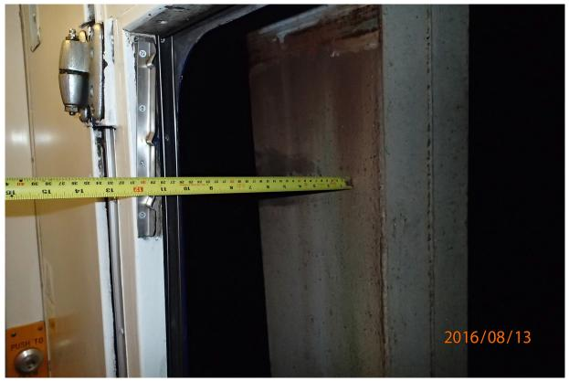
Figure 7: Static clearance to the gantry from the droplight window
