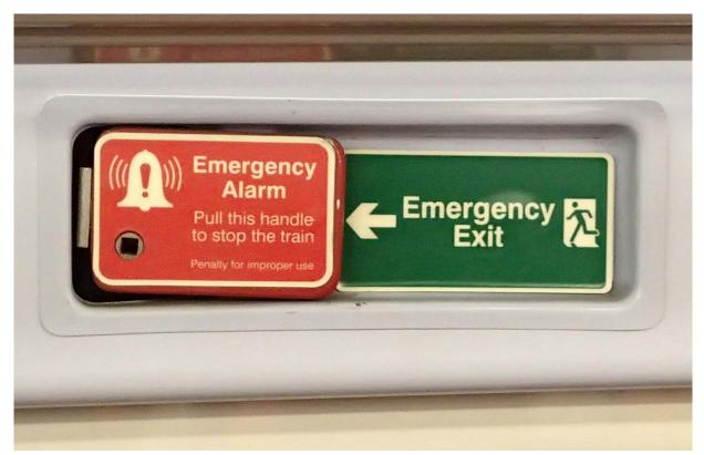
Figure 10: Emergency alarm on the Class 442 unit
