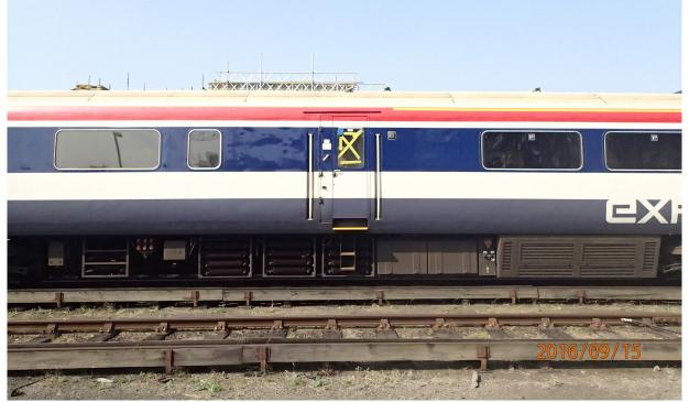
Figure 11: Class 442 unit with hazard tape applied to guard's droplight window
