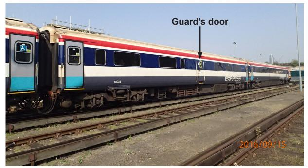
Figure 4: Middle carriage of a Class 442 unit showing guard's door (NB: the yellow tape on this door reflects a post-accident modification intended to discourage passenger use of the droplight window; see paragraph 111).
