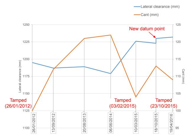
Figure 8: Graph of the lateral clearance and cant measurements since 2012
