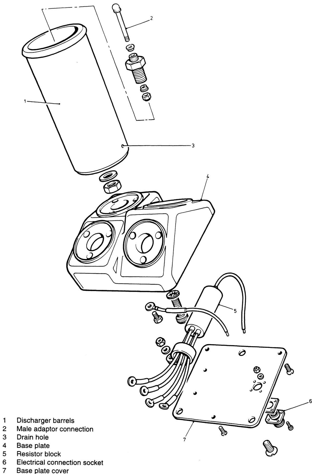
Fig 17 Smoke grenade discharger
