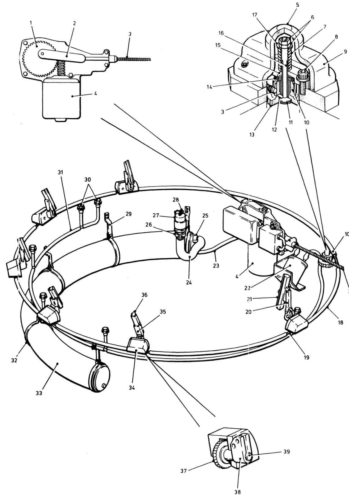
Fig 12 Washer/wiper system
