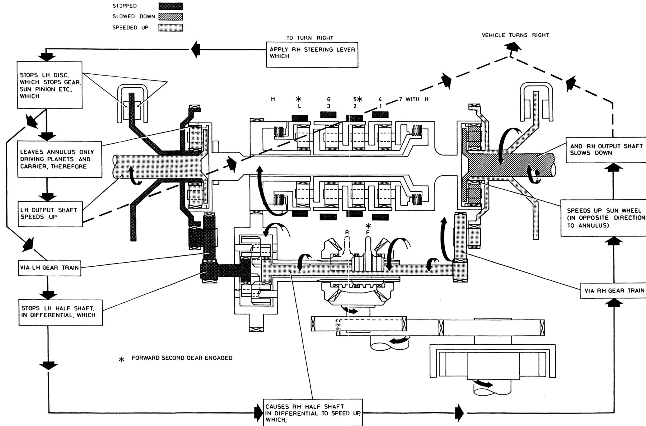
Fig 7 Steering operation - gearbox
