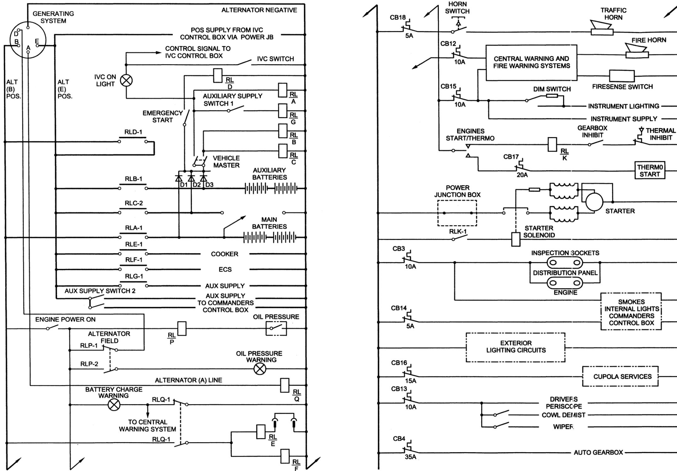
Fig 3 Distribution panel circuit - schematic
