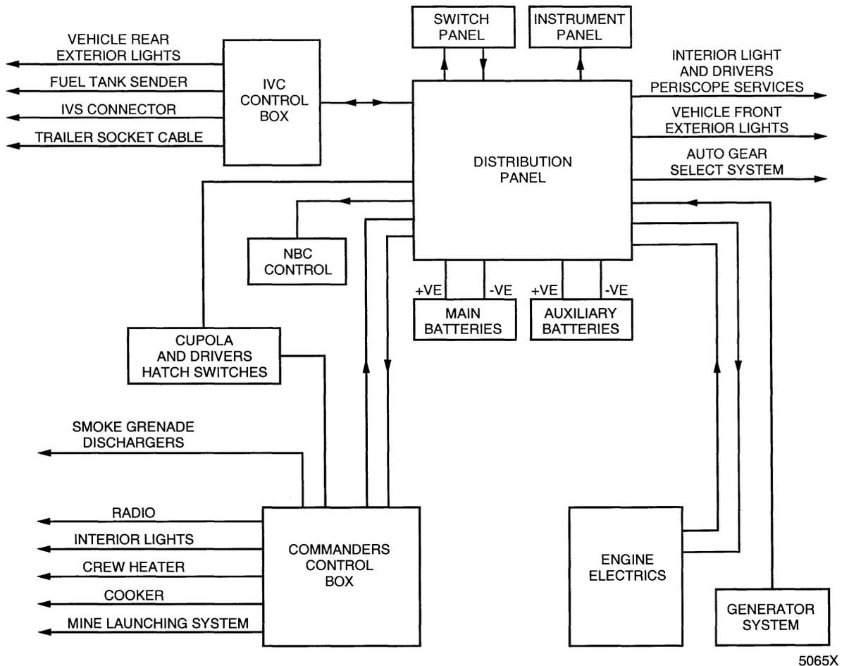
Fig 1 Vehicle electrical system - schematic
