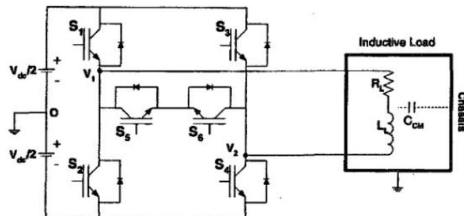
Figure 3.3: Schematic Diagram of the Proposed Single Phase Inverter Driving a Passive Load
