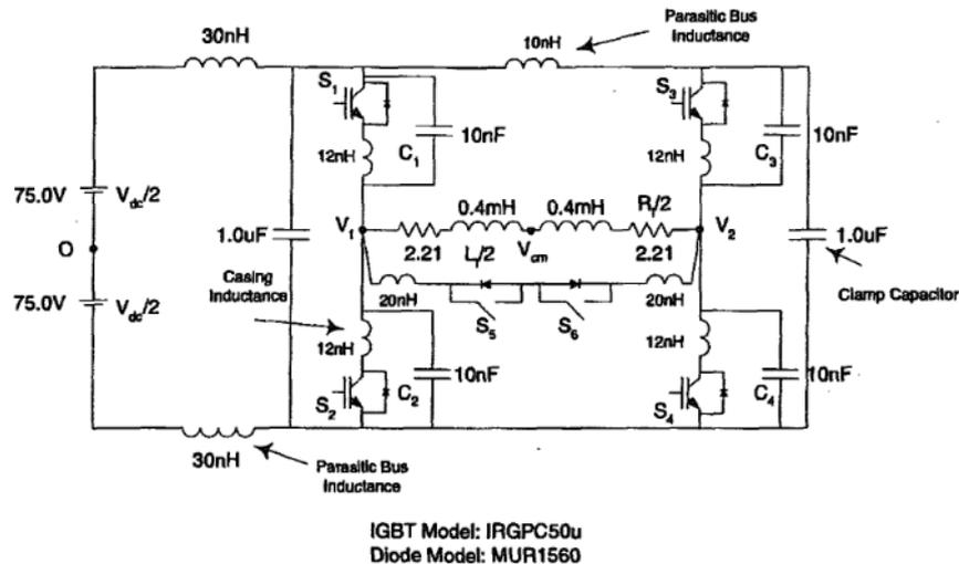
Figure 4.7: Simulation Model of Laboratory Prototype Inverter with Proposed Topology
