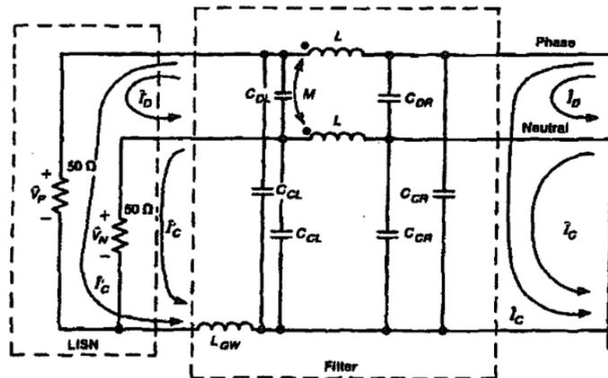
Figure 2.10: Schematic Diagram of a Typical EMI Filter Topology
