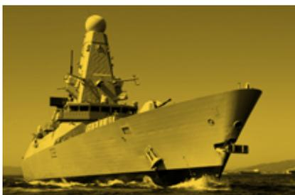
**Type 45 Power Improvement Programme (Project Napier)** – HMS DEFENDER will be completing deep maintenance only undertaken every six years and fitting a large number of additions and alterations which will ensure she remains current and capable. These include modifications to her power and propulsion plan under Project Napier's Equipment Improvement Plan and the fitting of additional and improved sensors that will mean she is one of the most up to date warships in the Fleet.
