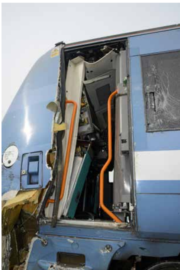
Figure 13: External damage to side of train 1K77
