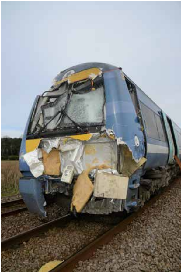
Figure 10: External damage to front of train 1K77
