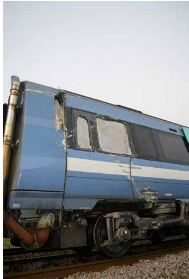
Figure 11: External damage to side of train 1K77
