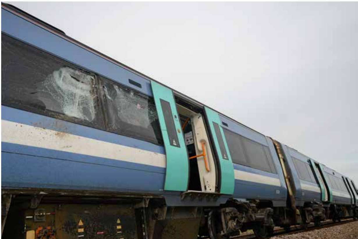
Figure 12: External damage to side of train 1K77
