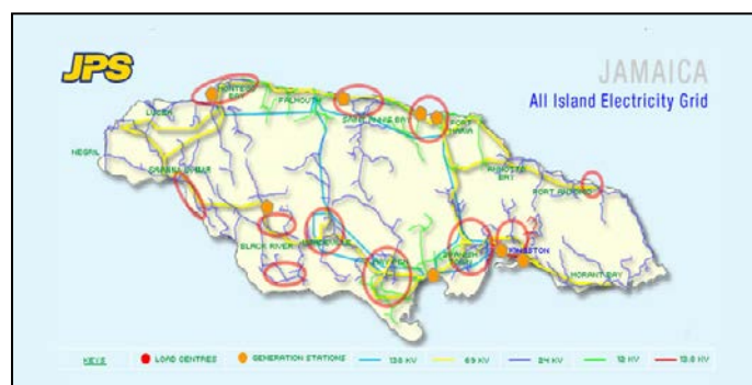
Figure 1. Locations of generation stations (orange pentagons) and load centres (areas circled in red). Medium to high voltage power lines of Jamaica's electricity grid are shown as follows: 12 kV power lines (light green), 13.8 kV (red), 24kV (blue), 69kV (yellow), and 138 kV (light blue). Source: Jamaica Public Service Limited.
