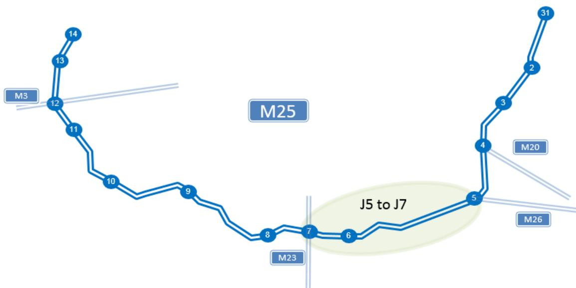
Although constructed as one Smart Motorway scheme, only J5 to J6 is all lane running, while the much shorter J6 to J7 remains four lanes plus hard shoulder on the link and three lanes plus hard shoulder through the junctions.
