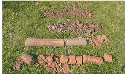
Core drilling samples are taken whenever there is a change in rock type or at 1 metre intervals
