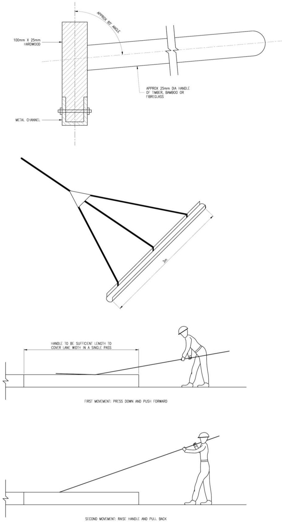
FIGURE 5.3: Scraping Straightedge
