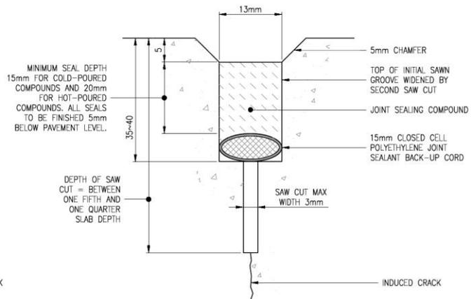
SEALED CONSTRUCTION GROOVE
