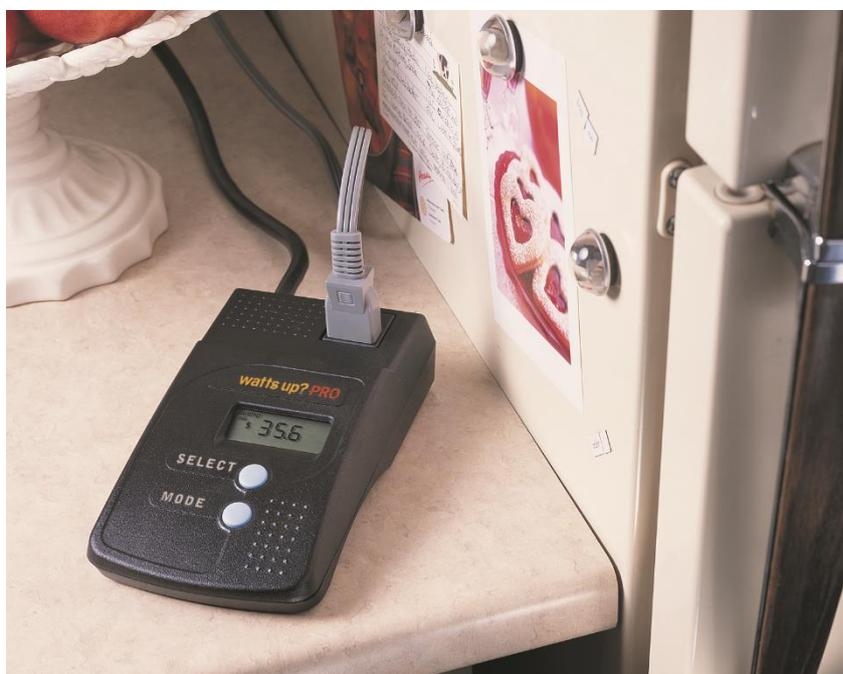
**Figure 1.** Watts Up PRO energy logger attached to refrigerator.
