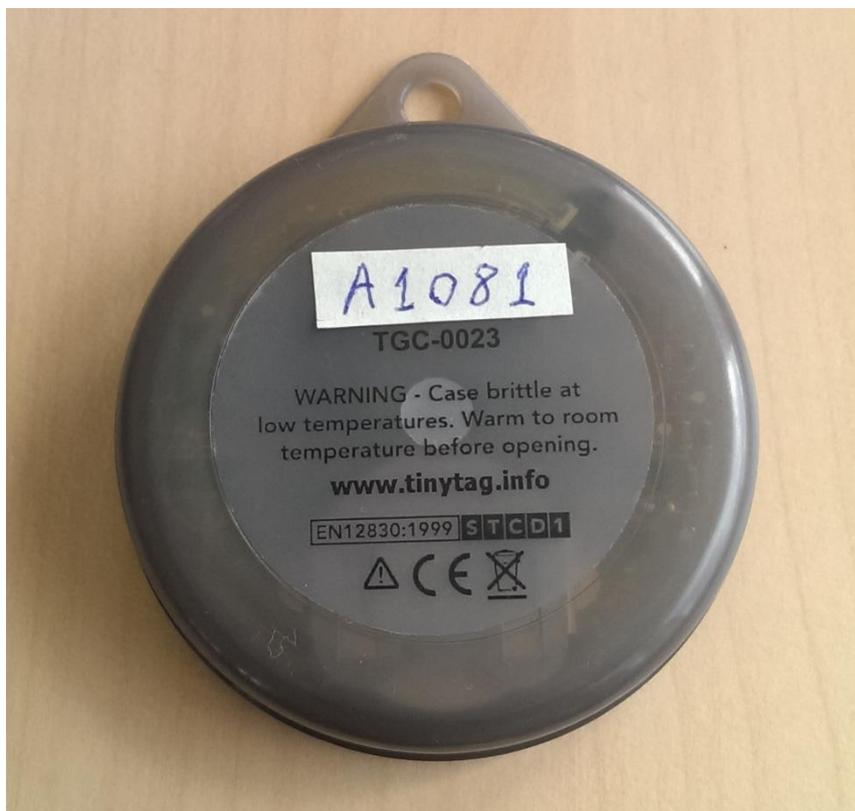
**Figure 2.** TinyTag transit 2 temperature logger.
