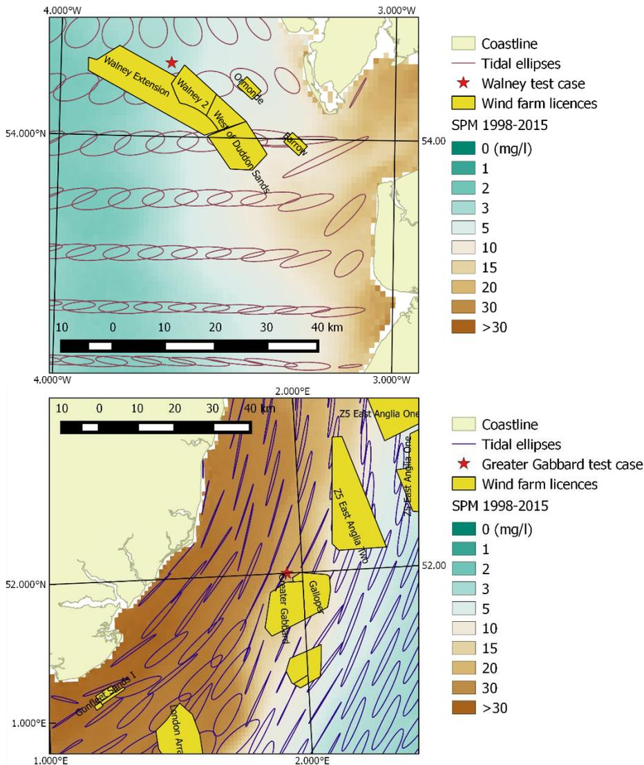
**Figure 9: Location of the windfarms used in the test cases: Walney 1 and 2 (top) and Greater Gabbard (bottom). The tidal ellipses indicate the direction of the tide. The red stars mark where the non-algal SPM values were extracted from.**
