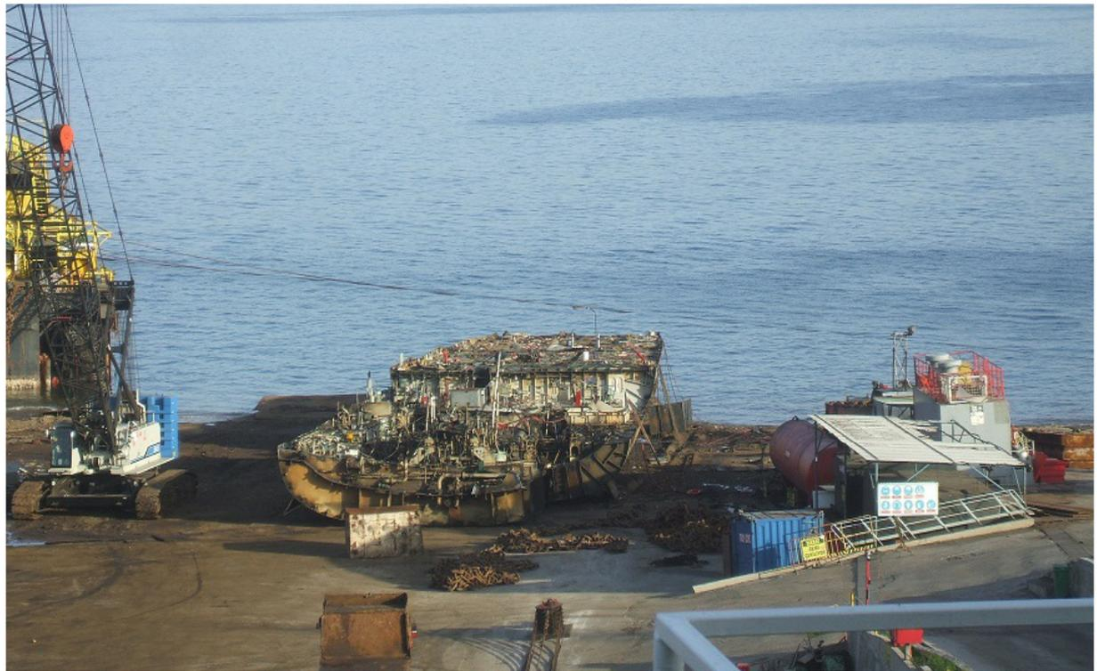
Final dismantling of the pump & engine room. The final recycling of the hull takes place completely on dry land where the remaining part of the keel is winched on to the landing area.
