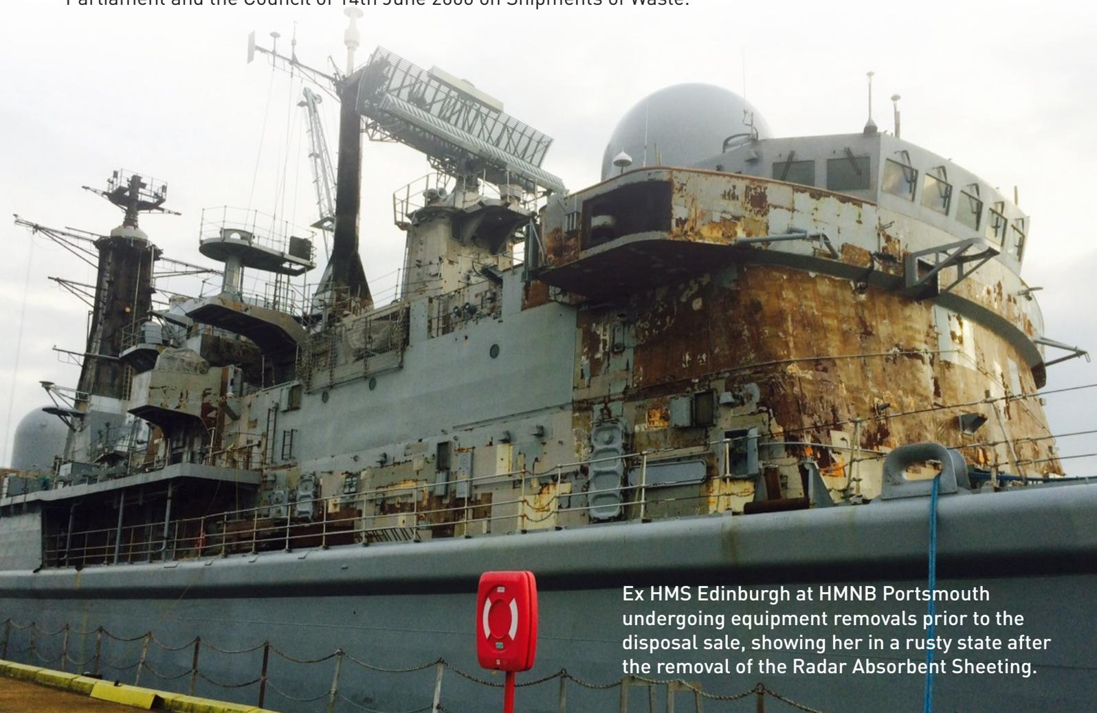
Ex HMS Edinburgh at HMNB Portsmouth undergoing equipment removals prior to the disposal sale, showing her in a rusty state after the removal of the Radar Absorbent Sheeting.
