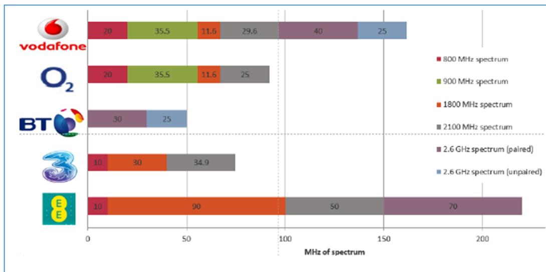
Figure 4: UK spectrum holdings after 4G auction and EE divestments in 1.8 GHz<sup>9</sup>
