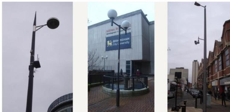
Figure 30: Outdoor street furniture small cells [Source: 3G4G Small Cells Blog]<sup>67</sup>
