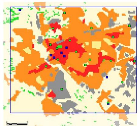
The total area within the blue polygon is 33km<sup>2</sup> (see right) and the size of the urban (red) and industrial (grey) clutter area is 6.4km<sup>2</sup>. Our analysis considered 29 sites for the multi operator configuration within the urban and industrial clutter area of Exeter and 17 sites for the single operator network. There were only three non-MNO sites which did not greatly impact the densification requirements.
