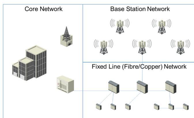
Figure 15: Simplified Private Radio/Fixed network architecture
