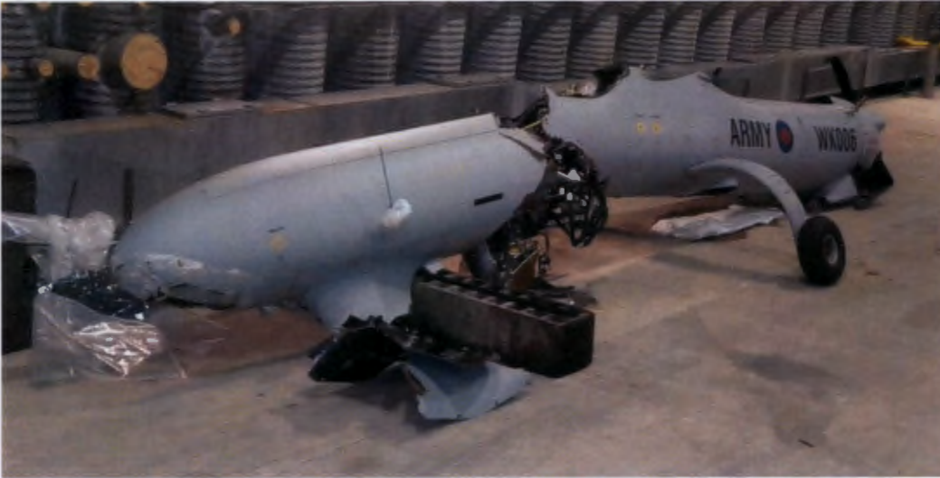
Figure 9 - Damage to UA (wing assembly removed).
