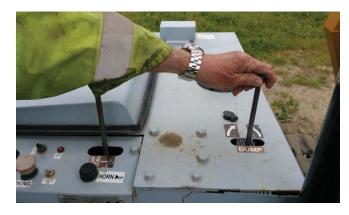
The Group's latest project – Reducing Unintended Movement of Plant – is about managing exposure to consequential risks, where inadvertent operation of a control, such as a switch, lever, pedal etc, has caused unintended machine movement resulting in, in several cases, serious injuries or fatalities.
