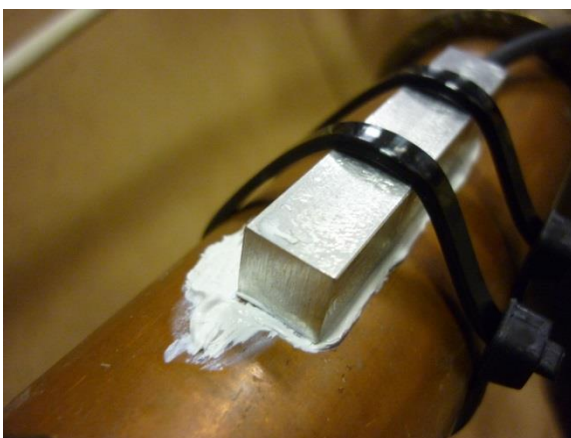
Figure 30: Surface temperature sensors with thermal paste
