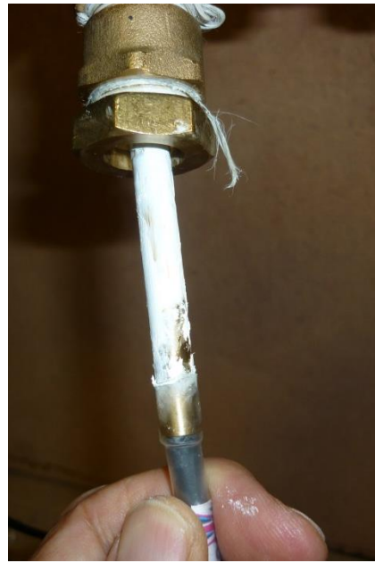
Sensor smeared with thermal paste prior to insertion into pocket
