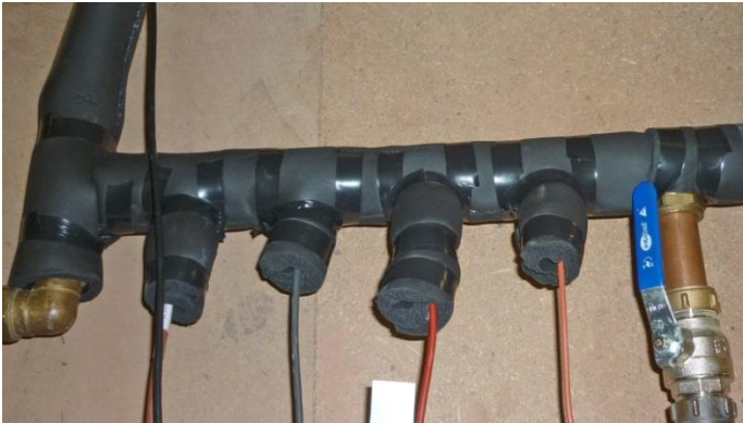
Figure 27: Sensors mounted in pockets (insulated and uninsulated, with and without paste)
