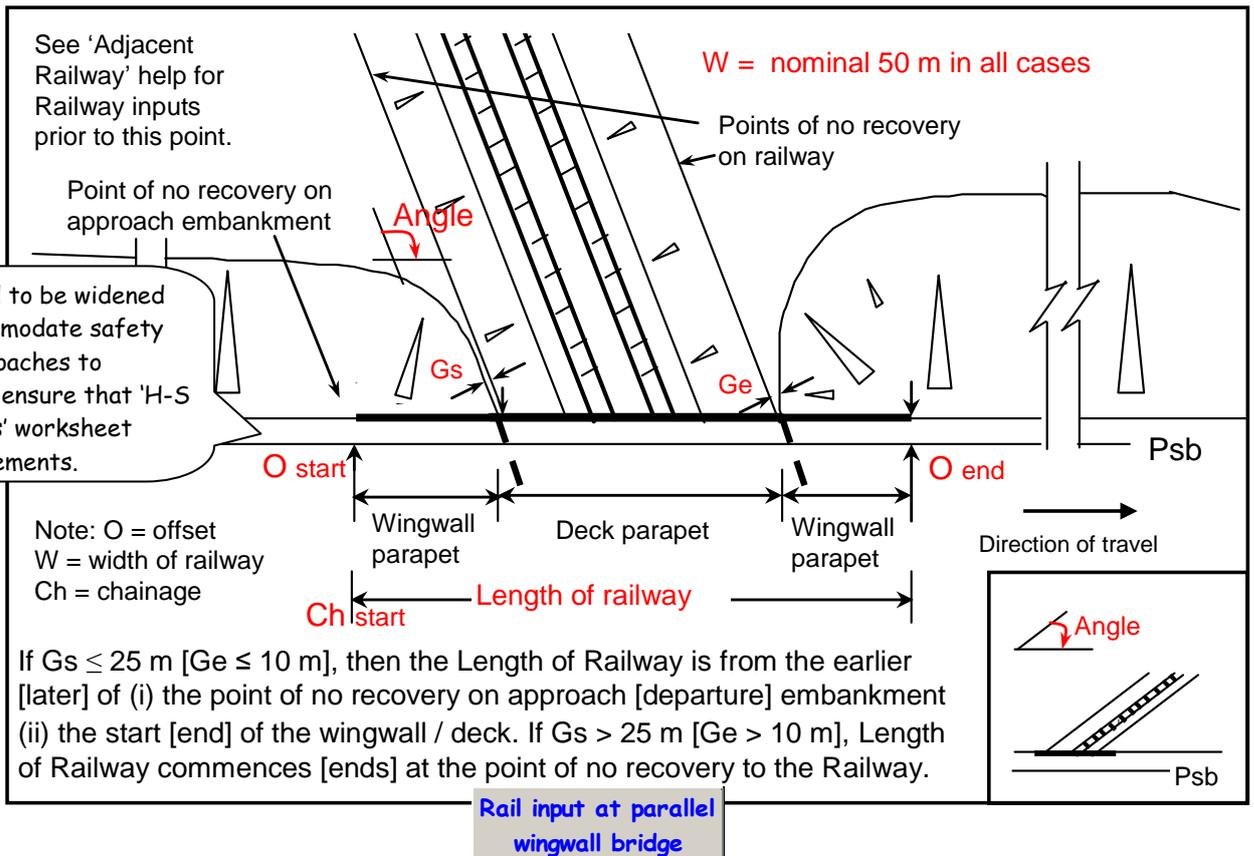
**Figure 5.14 (d) Railway crossing under Road at structure with parallel wingwalls**
