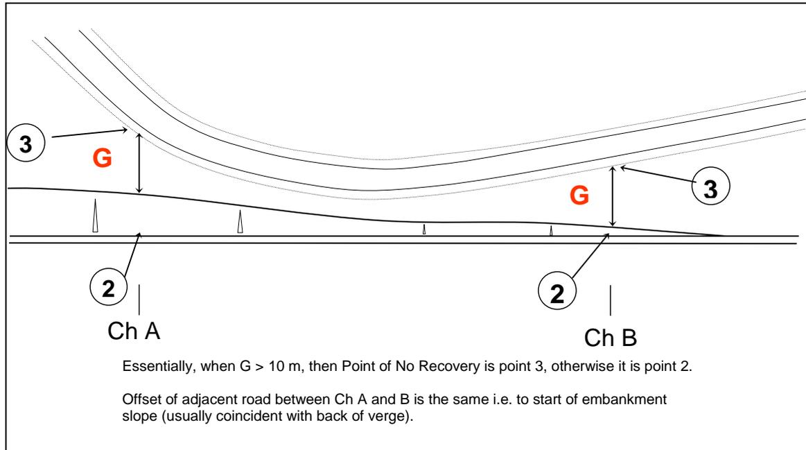
**Figure 5.14 (c) Point of No Recovery for Parallel Road / Rail situation (2)**
