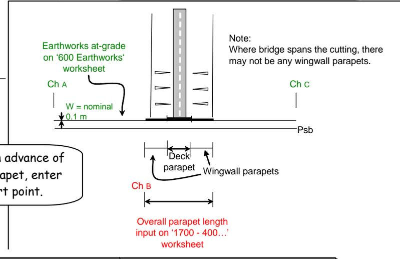
If the 25 m extends in advance of the actual start of parapet, enter the actual parapet start point.
