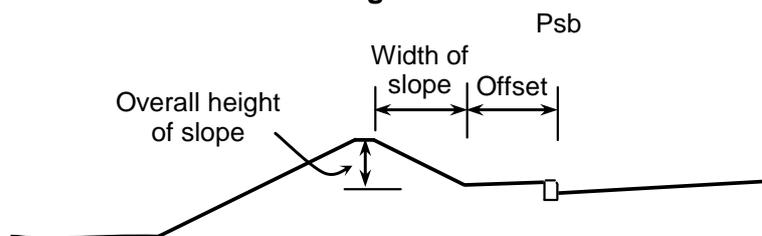
**Fig 5.3.3 (c) Multiple slopes where height of false cutting is  $\geq 2.5$  m**
