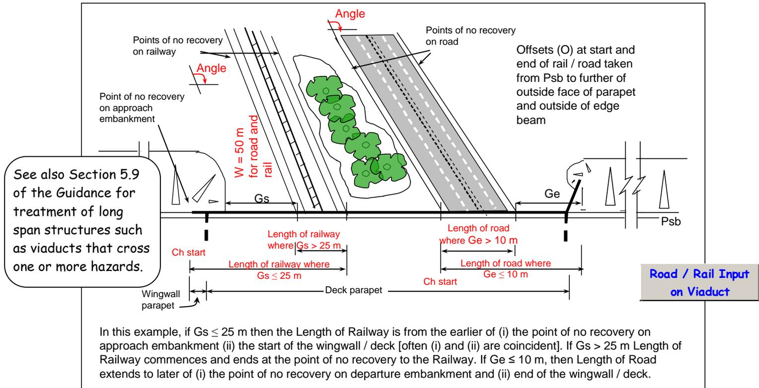
**Figure 5.15 (d) Viaduct with Road and Railway crossing under the Road**
