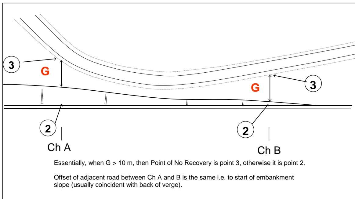
**Figure 5.15 (c) Point of No Recovery for Parallel Road situation (2)**
