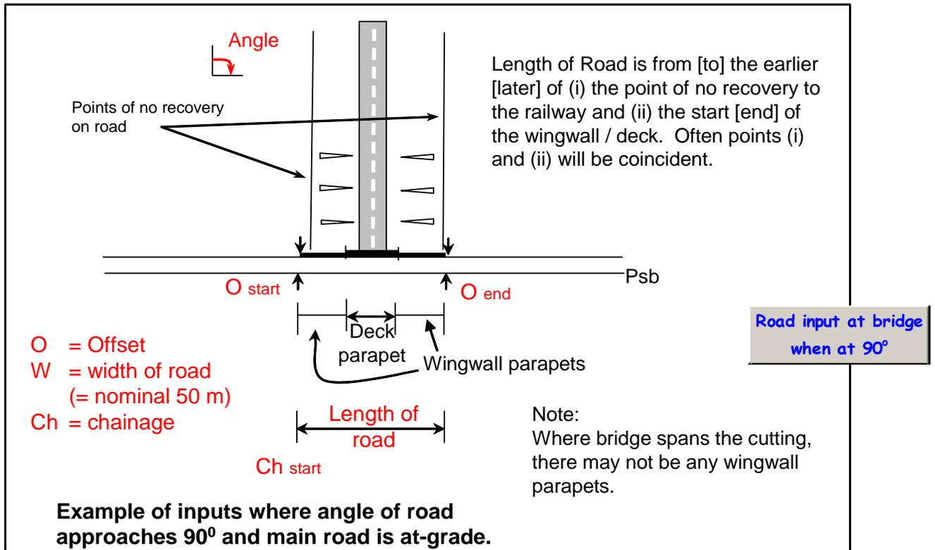
**Figure 5.15 (g) Road crossing under Road where at-grade and or at 90°**
