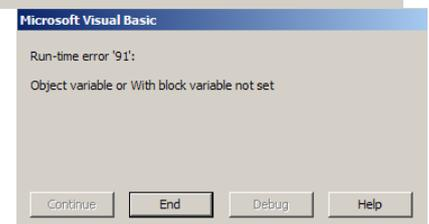
(f) This will be returned if the % LGV and or % MGV value has not been entered on the Basic (Common) Details worksheet. The programme is then unable to complete the calculation and may lock up.
