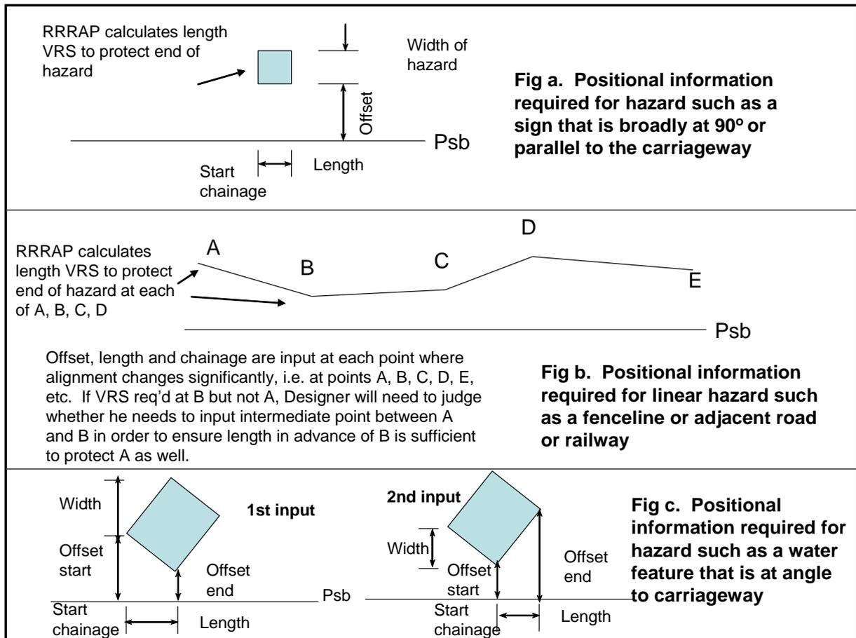
**Fig 1-4 Positional information required by RRRAP in order to calculate VRS requirements** – note that this gives typical details; further particulars are contained within each of the relevant sections.
