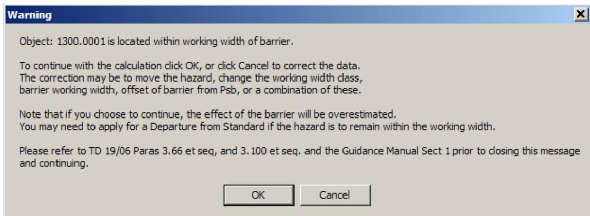
If the OK button is pressed without the data being corrected or changed, the Collation of Data worksheet will highlight the data line that contains the information as shown below.
