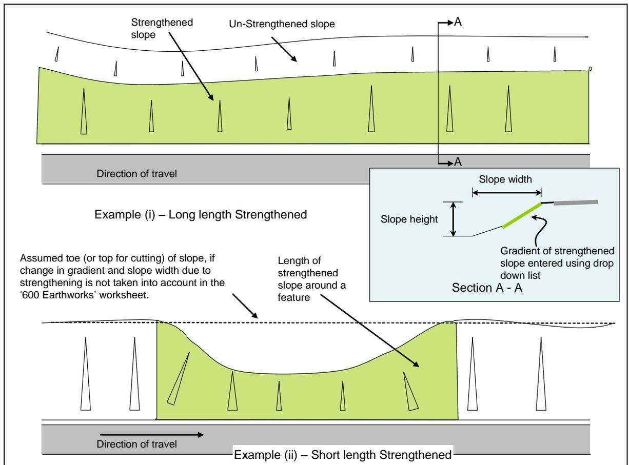
**Figure 5.10 (a) Strengthened Slopes**
