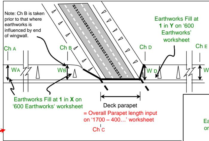
Parapet details are entered in the 1700 - 400 Structures - Parapets worksheet as indicated in these helps. See also the OH's Road and OH's Rail worksheets and Helps for how to input details relating to road and or railways.
