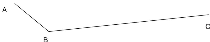
5.2.4 If there is a drainage item such as a drainage lagoon that is at an angle to the carriageway, e.g. as shown below, such that the difference in offset at A and B is significant, then the hazard should be entered twice, once to pick up chainage, offset and width at point A and second to pick up chainage, offset and width at point B. Where the offset at A and B are broadly similar, the data entered would be chainage A, nearer offset of A and B, and max width of hazard.
