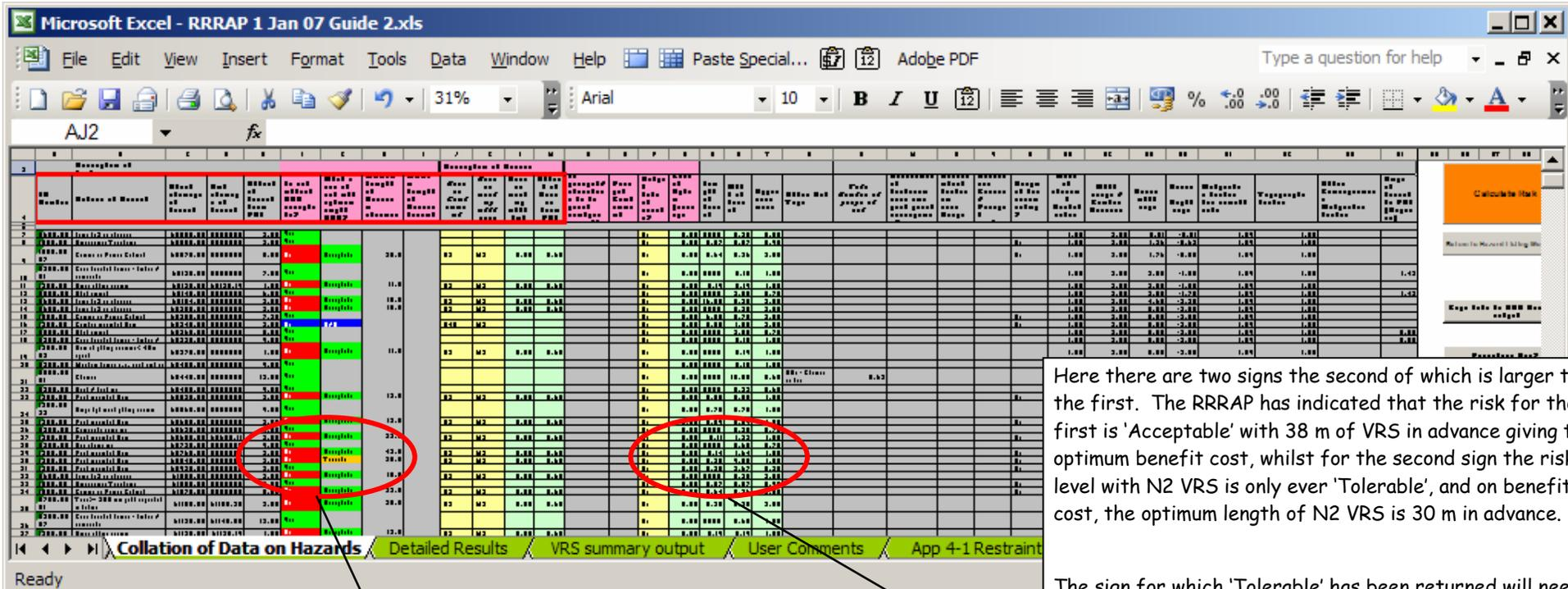
Here there are two signs the second of which is larger than the first. The RRRAP has indicated that the risk for the first is 'Acceptable' with 38 m of VRS in advance giving the optimum benefit cost, whilst for the second sign the risk level with N2 VRS is only ever 'Tolerable', and on benefit cost, the optimum length of N2 VRS is 30 m in advance.
