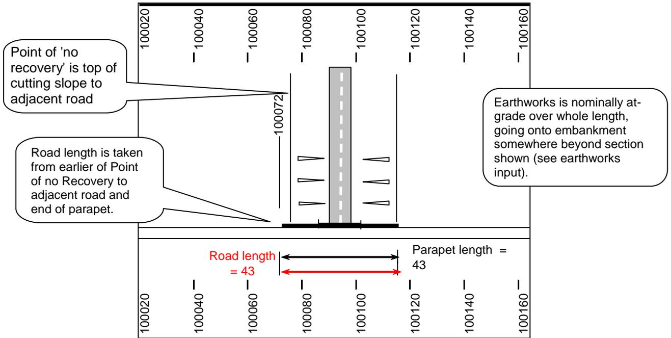
**Figure 5.9 (e) Adjacent Road crossing at-grade and or at around 90°
