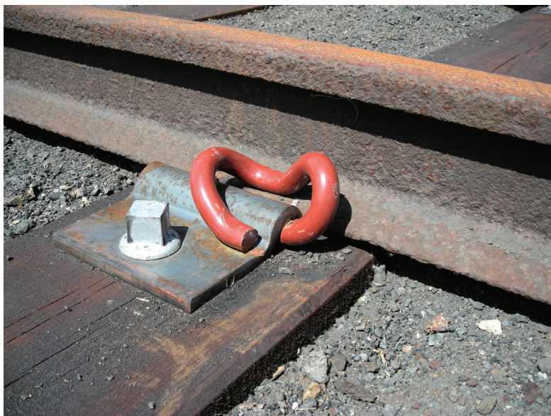
Figure 9.5 Pandrol clip PR401A with BS75R rail on timber sleepers
