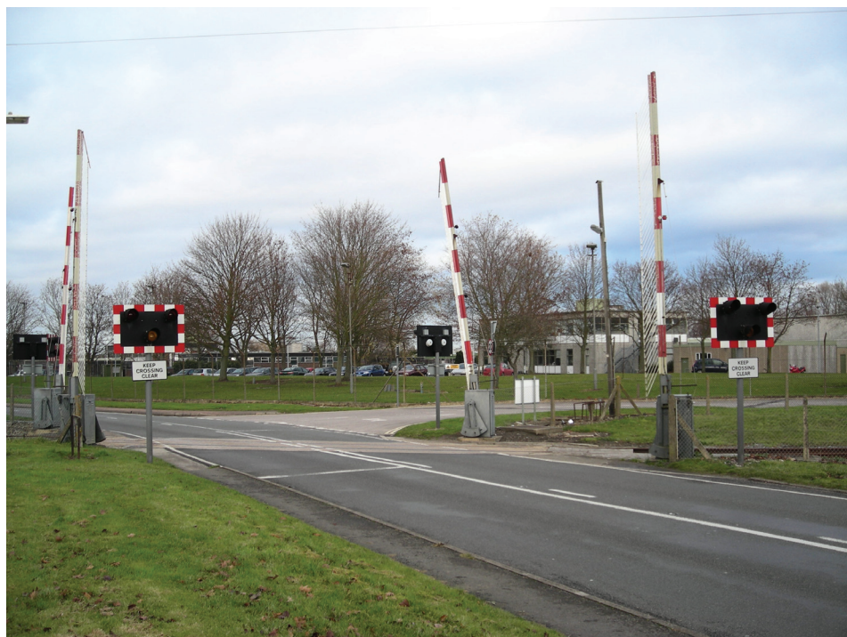
Figure 10.7 Full barrier level crossing, manually initiated.
