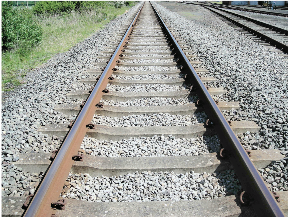
Figure 7.5 Plain line track – BS113A rail on concrete sleepers
