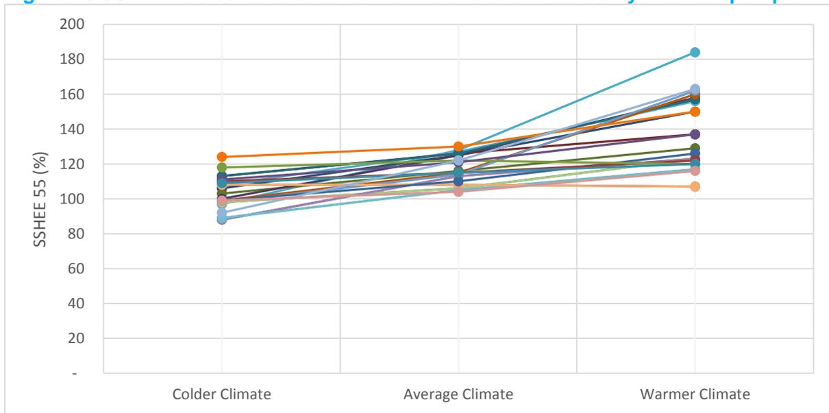
The average SSHEE at 55°C for air to water heat pumps at average climate conditions was 119% and the maximum and minimum 133% and 108% respectively. The SSHEE value gives the performance in primary energy terms and converting these to performance in terms of delivered electricity by multiplying by 2.5/100 implies approximate seasonal performance factors (SPF) ranging from 2.6 to 3.75 which are all greater than the minimum SPF of 2.5 required for renewable energy.
