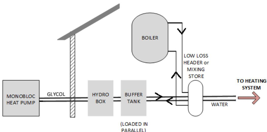
**Figure 9 Split hybrid heat pump providing space heating and domestic hot water pre heating**
