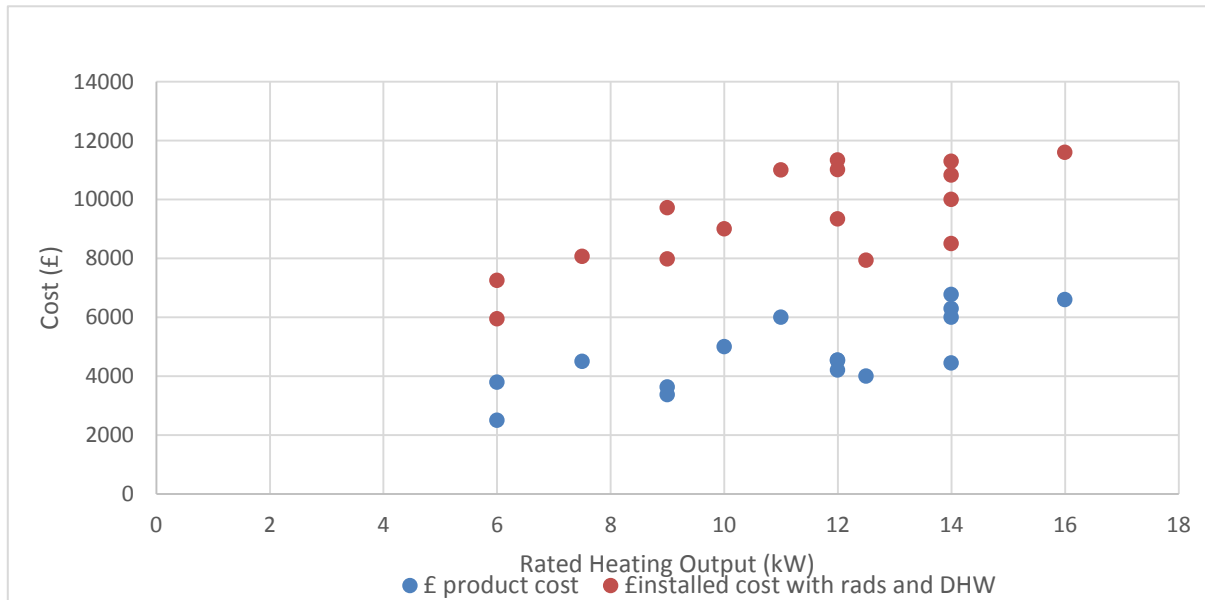
Figure 24 Range of air source heat pump product costs and total installed costs by capacity
