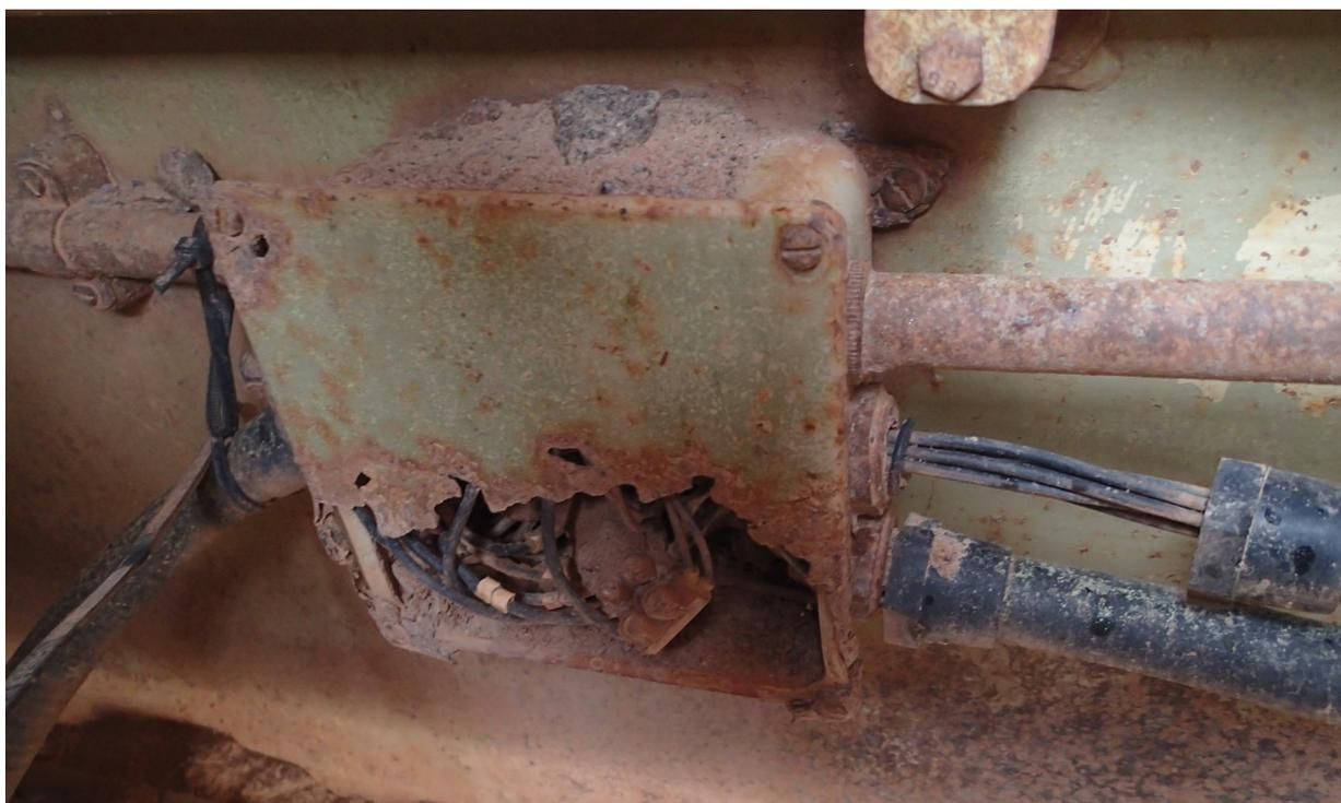
Figure 16: Wiring junction box beneath 'spider' switch
