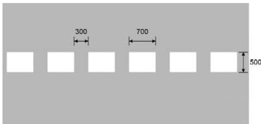
Figure 2.1.2: TSRGD diagram 1003.3
