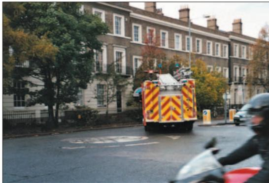
Photo 3.10.2: Fire engine negotiating mini-roundabout
