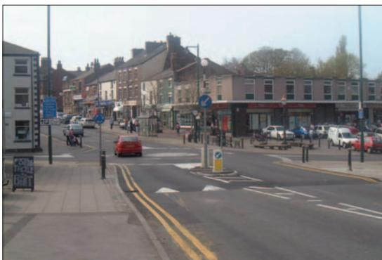
**Photo 3.6.3: Mini-roundabout on raised junction**
