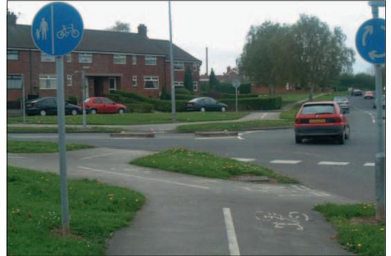
Photo 3.11.2: Mini-roundabout with off-highway cycle facilities
