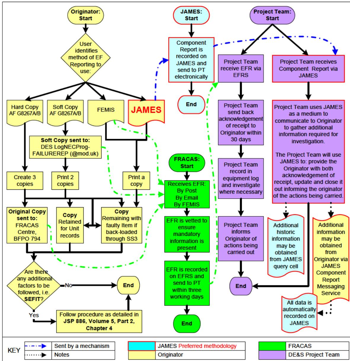
**9. Available EFR Options.** There are currently four different options available to the originator to report an Equipment Failure. Three of these are Electronic submissions, with a fourth option as a manual form for more complex EF Reports and lack of facilities. The electronic submissions are the preferred options and are to be used in all circumstances; the manual may only be used by exception only. In order of preference:
