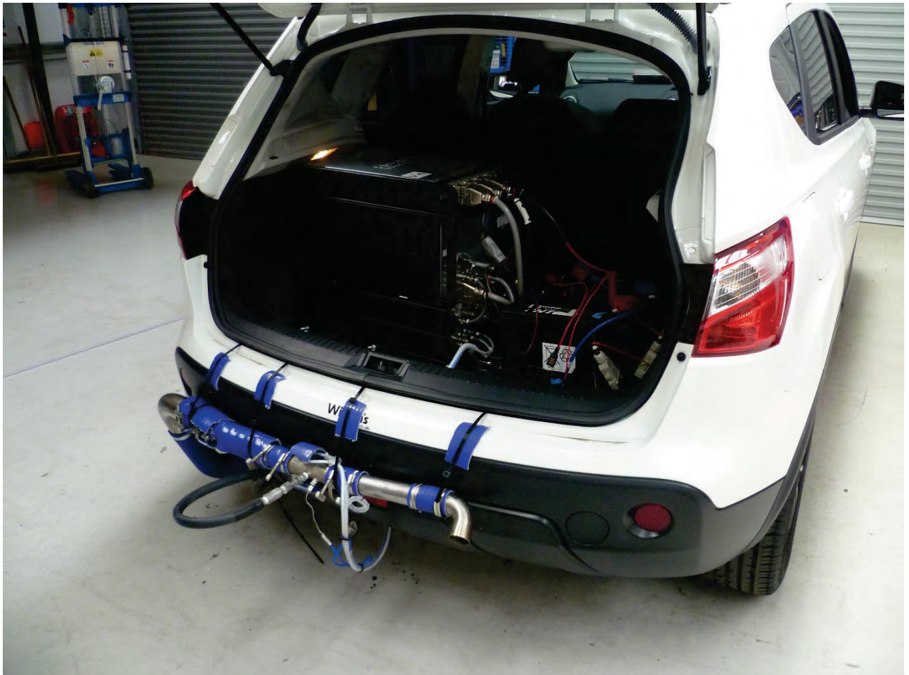
Figure 4-1 Portable emissions measurement system (PEMS) installed in a test vehicle
