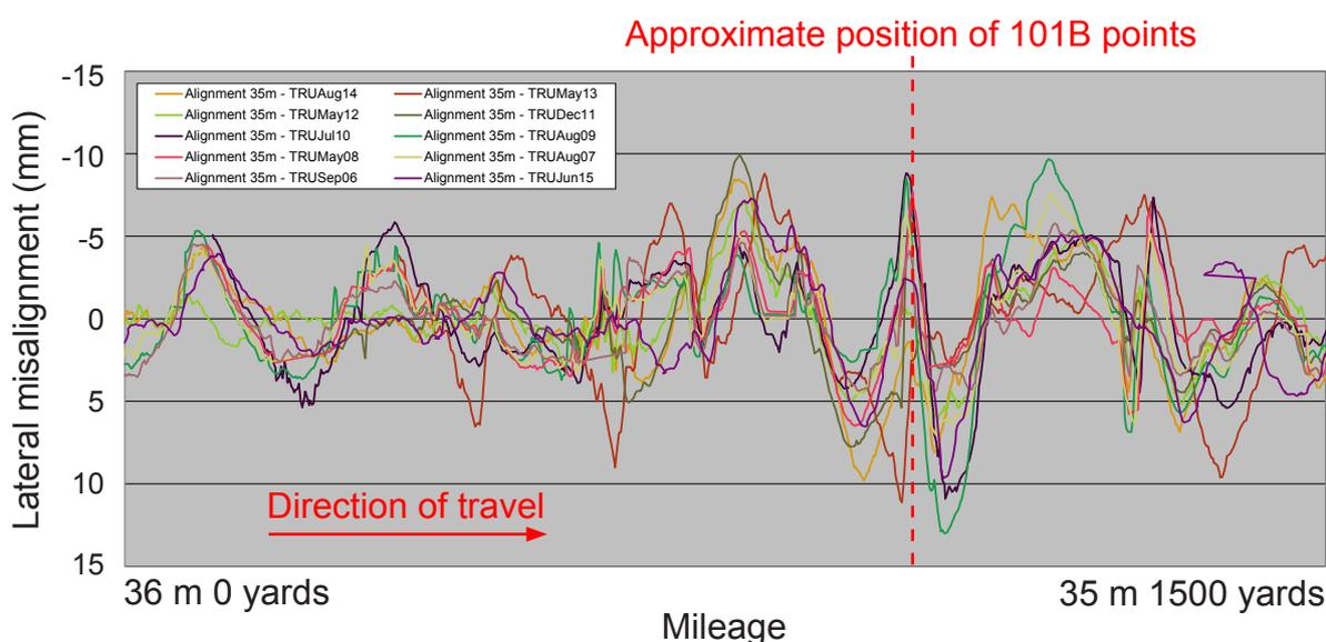
Figure 15: Traces of track alignment 2006 to 2014 for up line at 35 miles 1500 yards to 36 miles 0 yards
