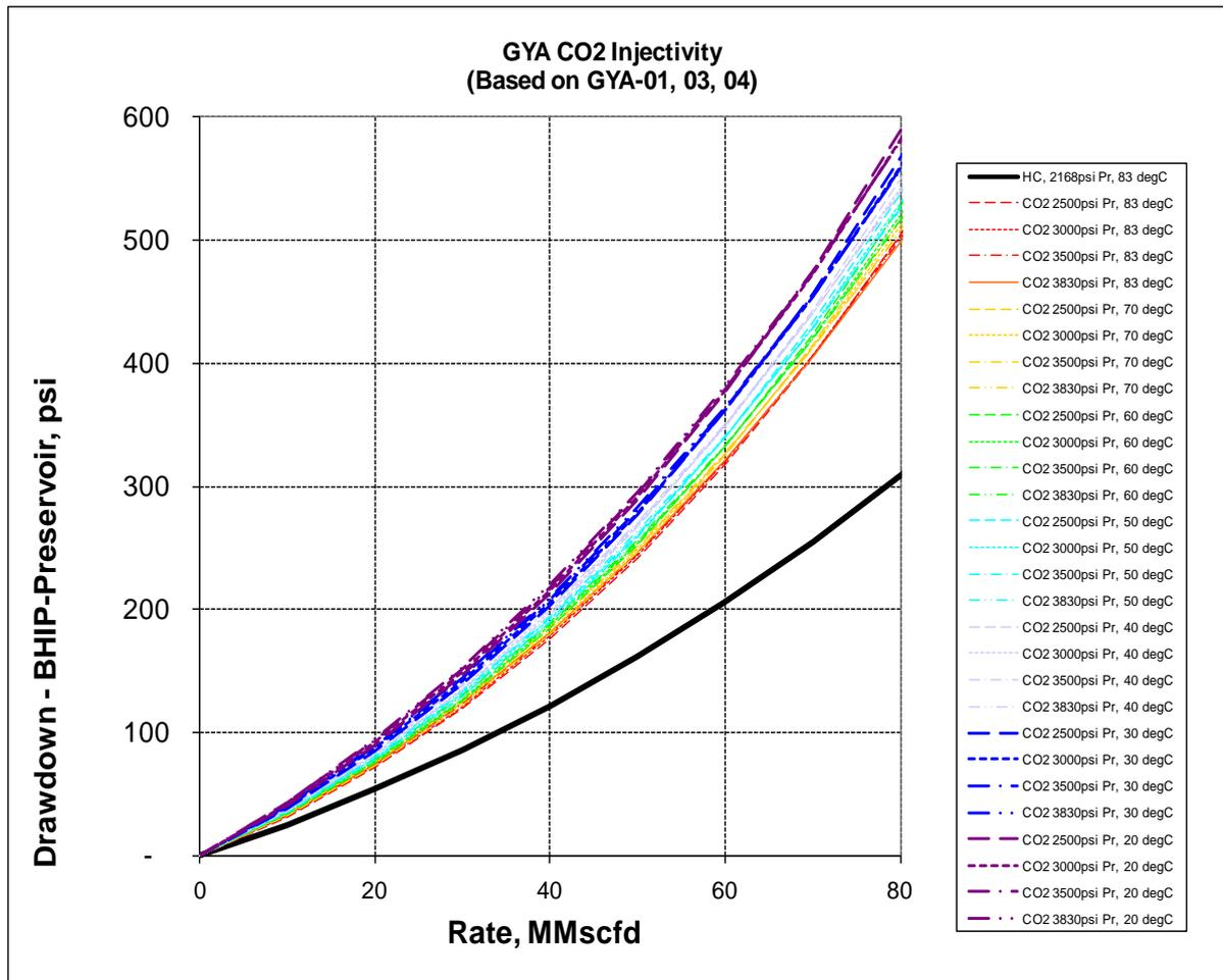
Figure 7-9: CO<sub>2</sub> injectivity vs hydrocarbon productivity (GYA01, GYA03 and GYA04).
