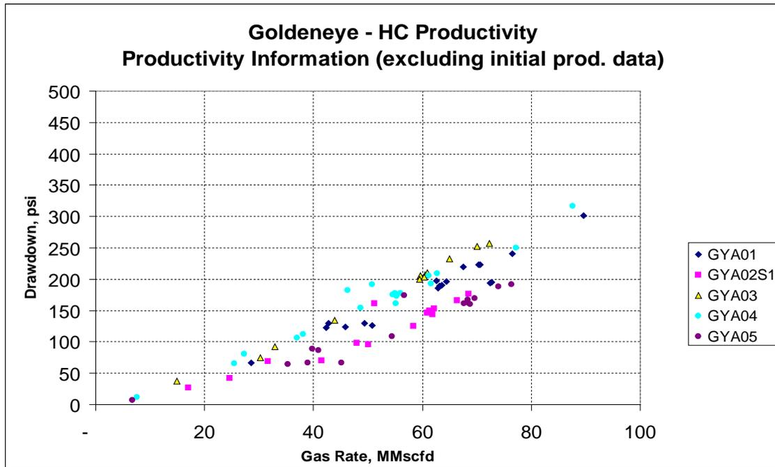
Figure 7-8: Productivity per well during long term production phase.
