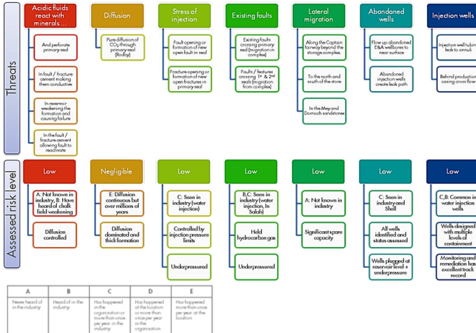
Figure 2-5: Bow-tie diagram for containment risks.
