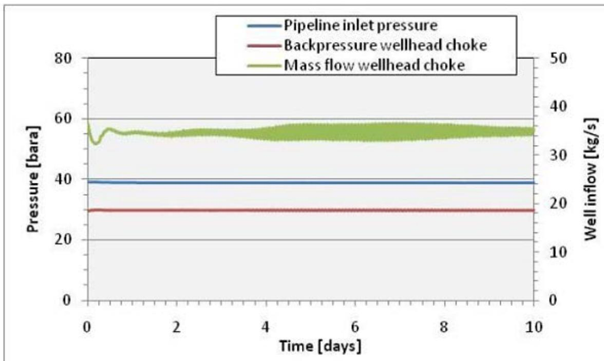
Figure 8-2: Stable behaviour: Two phase at 125 tonnes/hour.
