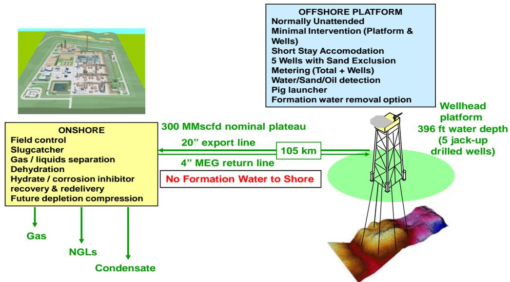
Figure 4-8: Goldeneye field hydrocarbon development plan.
