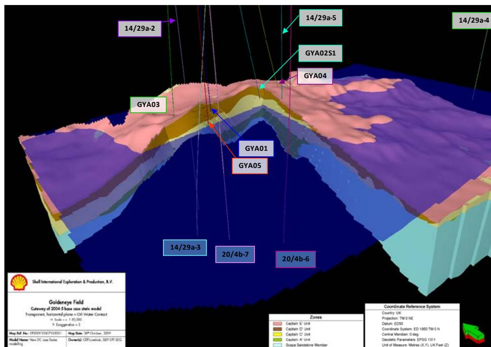
Figure 2-1: Goldeneye reservoir cross-section.
