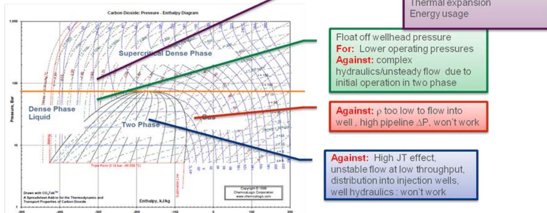
Figure 8-1: Modes of pipeline operation
