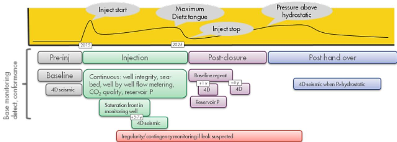
**Figure 10-1: Schematic of the monitoring plan. The vertical axis on the schematic represents risk of significant irregularity.**
