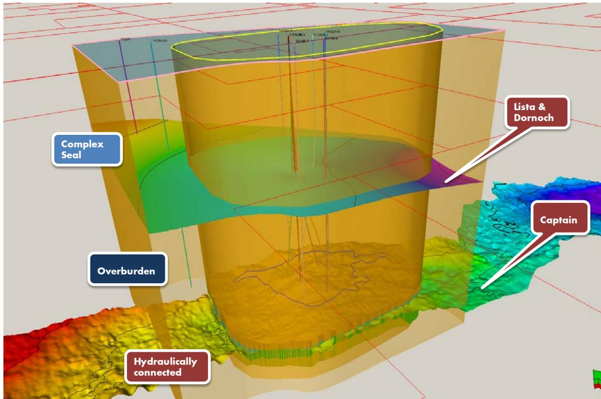
Figure 4-3: Schematic representation of the Goldeneye *storage site* and *storage complex* – not to scale.
