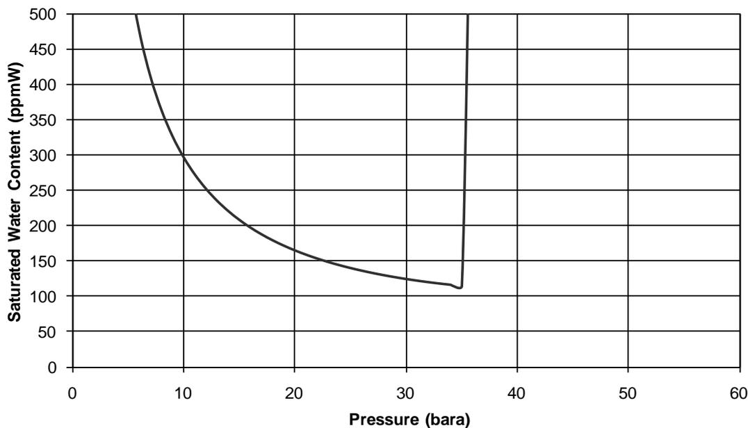
Figure 8-4: Saturated water content of CO<sub>2</sub> at 1°C.
