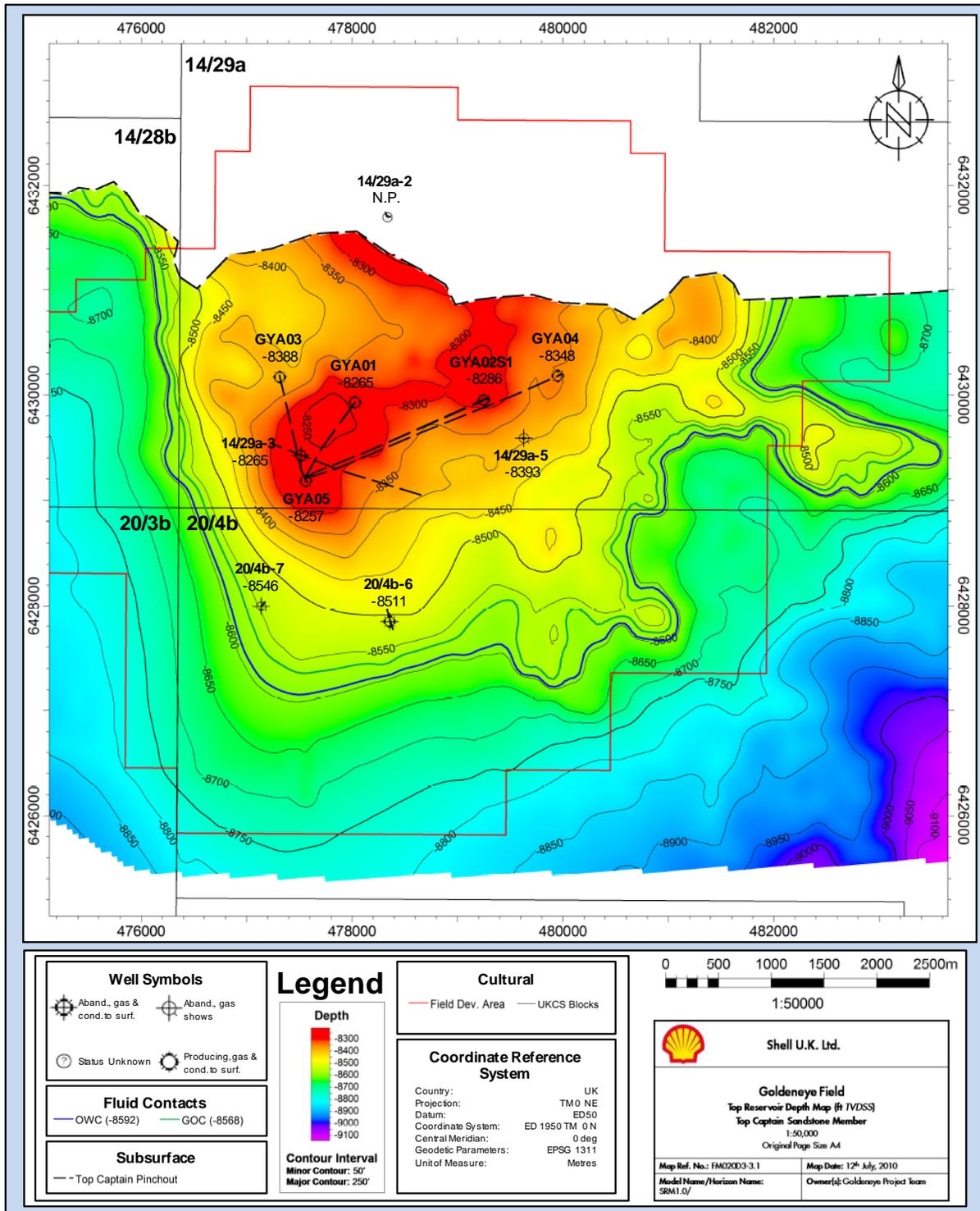
Figure 4-7: Goldeneye field top structure map – reference case.
