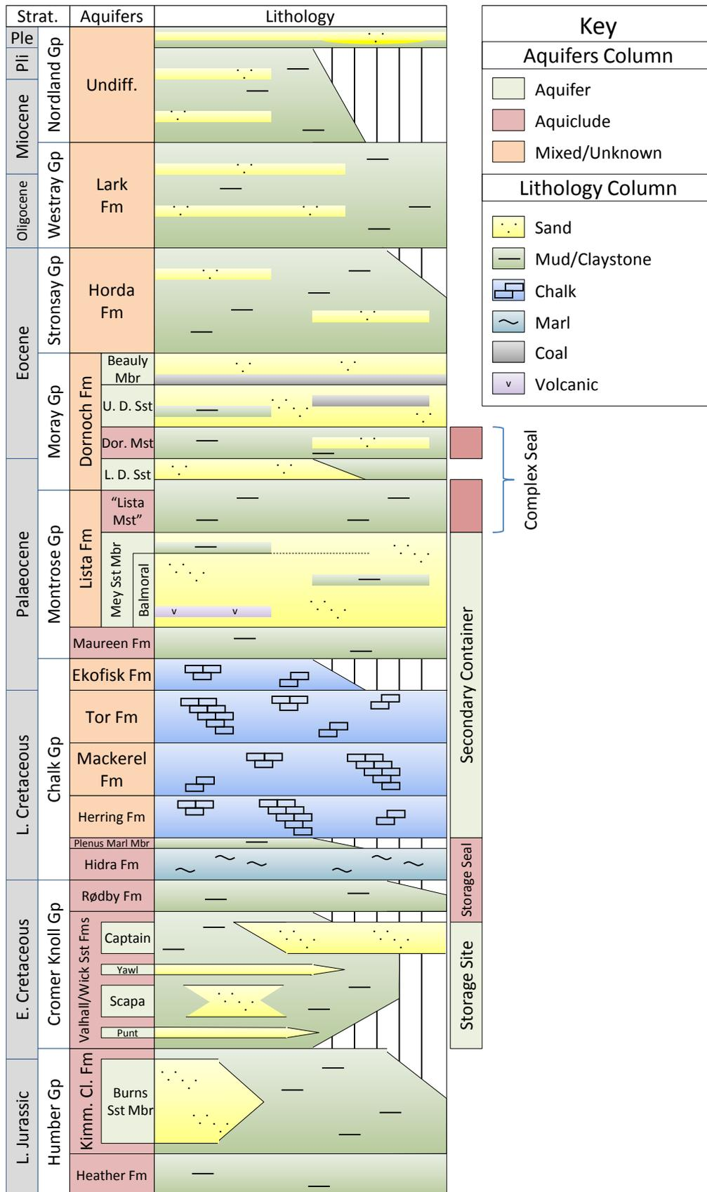
Figure 4-1: Generalised stratigraphy of the Goldeneye storage complex.
