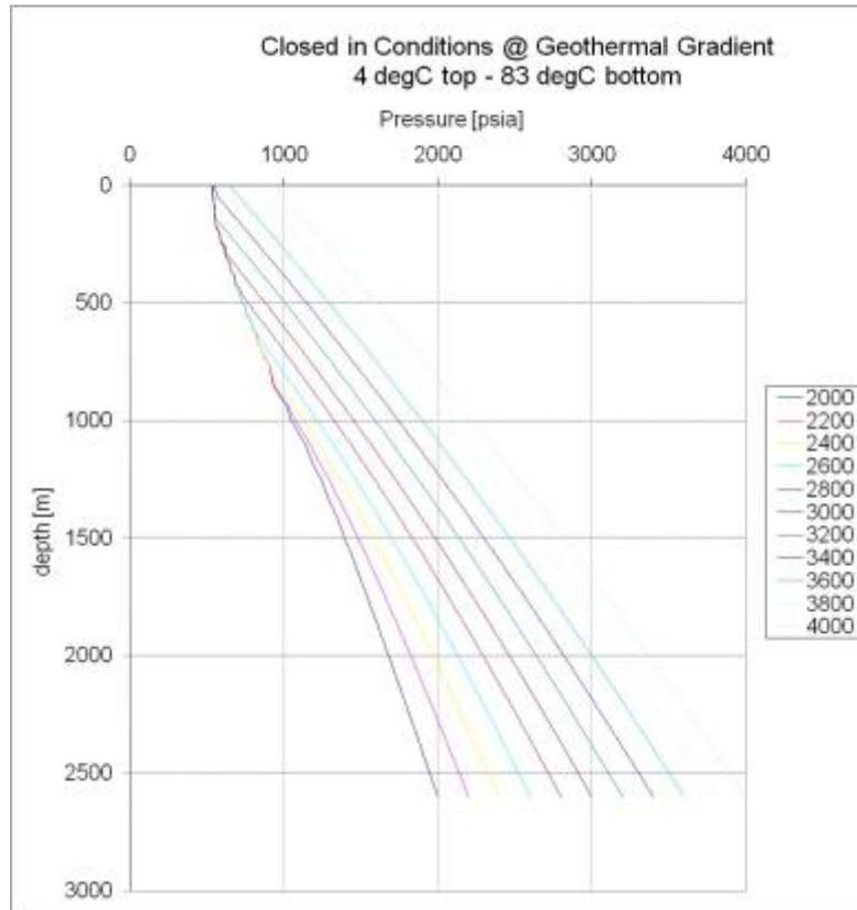
Figure 7-2: Pressure profile in a closed-in well (at geothermal conditions).
