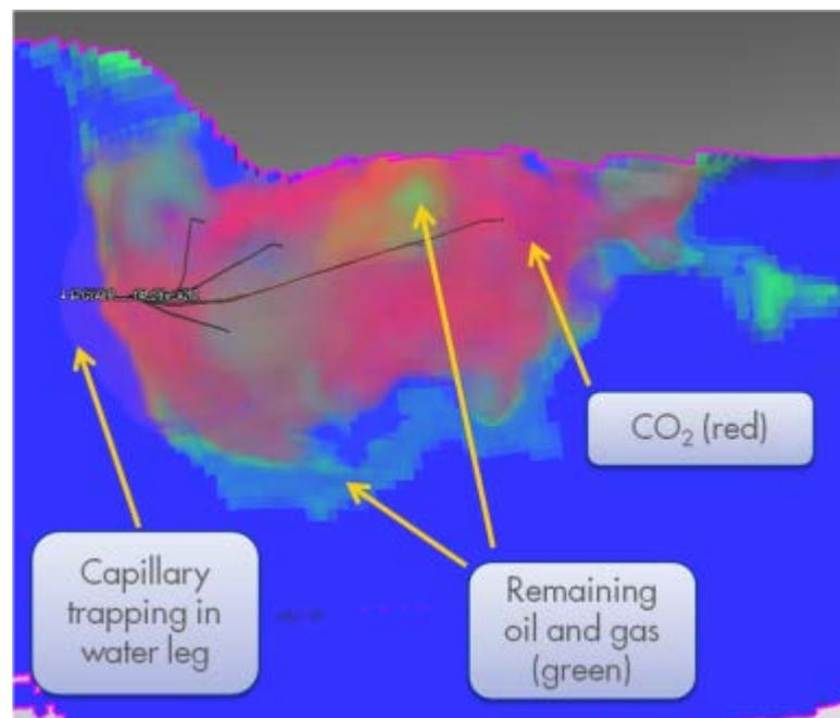
**Figure 2-2: CO<sub>2</sub> plume after injection.**
