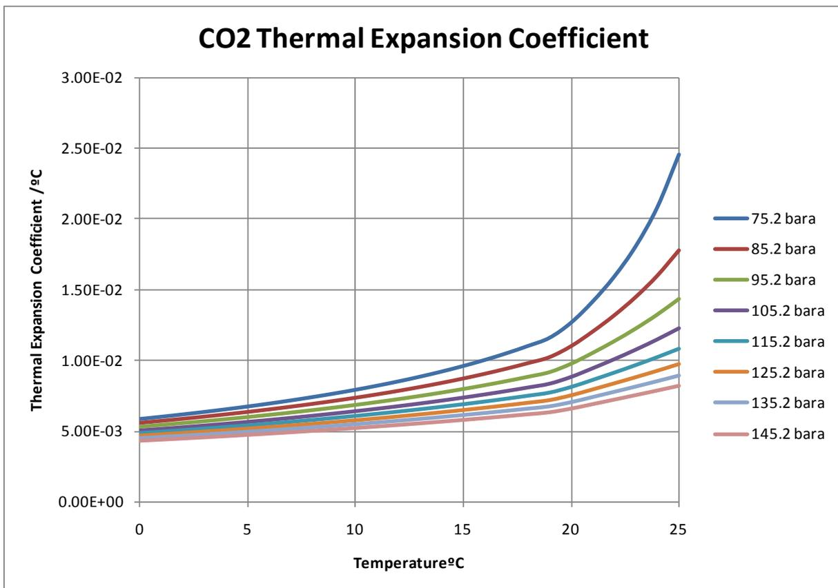
Figure 8-9: Dense phase CO<sub>2</sub> expansion coefficients.
