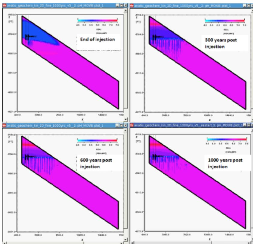
Figure 9-7: pH evolution through time. Colour scale runs from pH 4.0 to 7.5.
