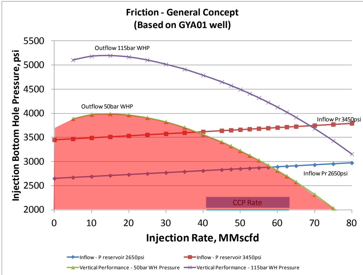
Figure 7-3: Outflow curves for the friction concept.
