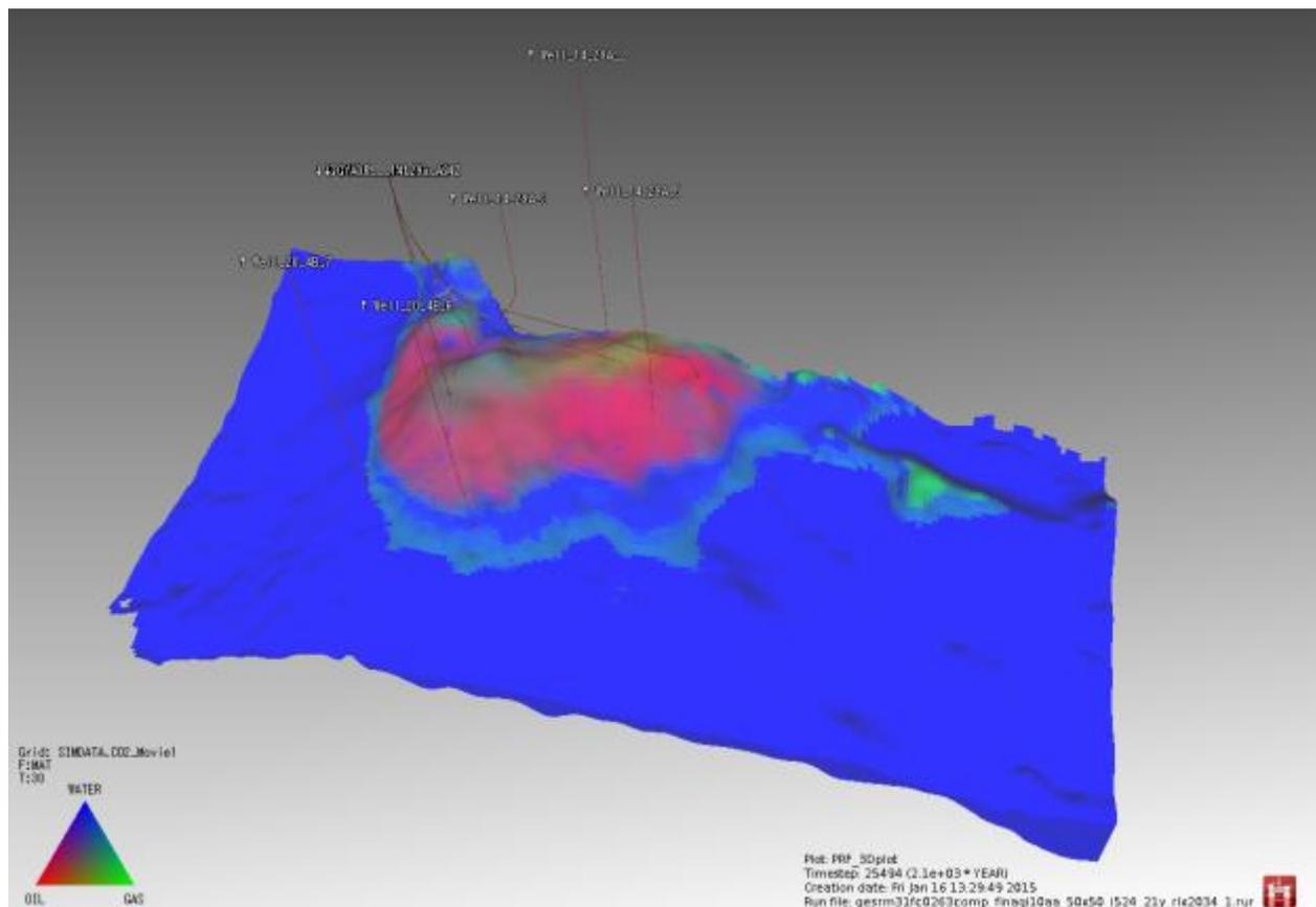
**Figure 12-1: Modelled distribution of CO<sub>2</sub> at the end of injection**
