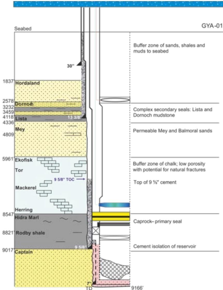
Figure 9-12: Example of Goldeneye injection well showing proposed injection completion and location of primary and secondary barriers.
