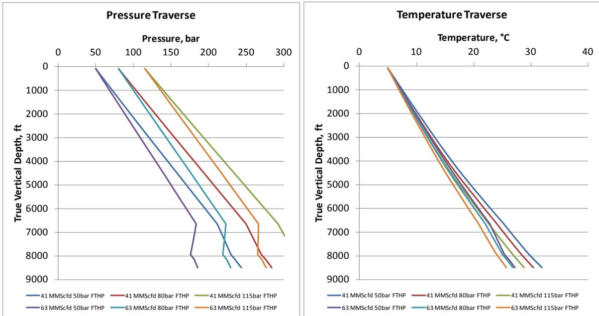
Figure 7-4: Pressure and Temperature predictions under steady state
