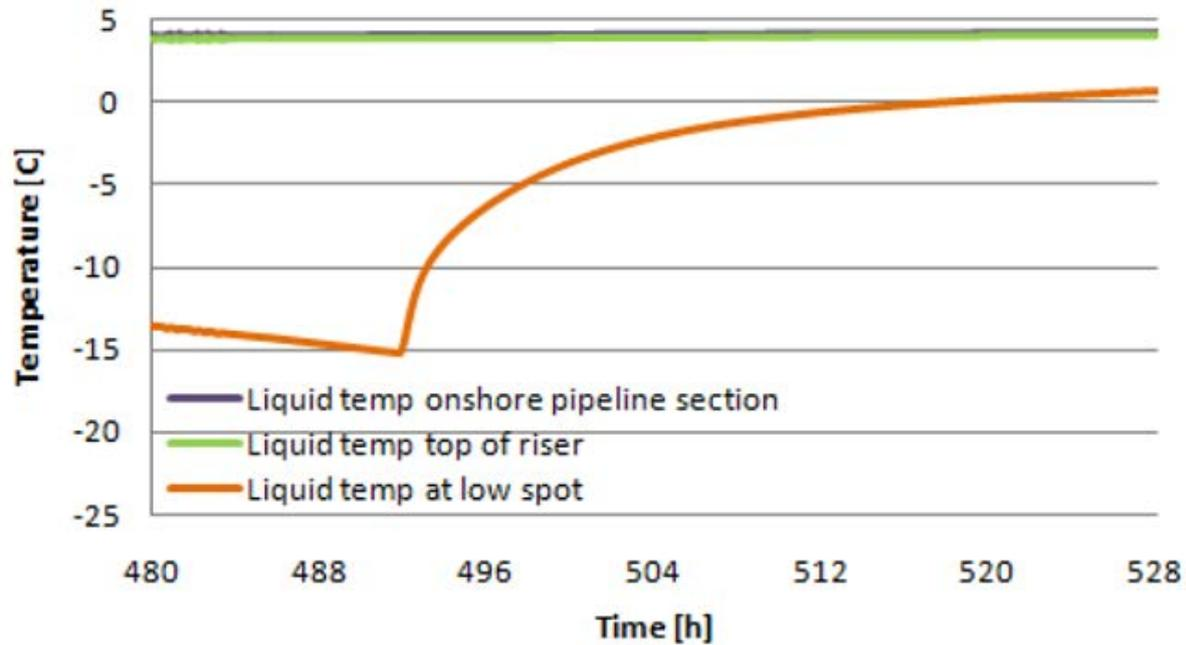
Figure 8-5 Pipeline fluid temperature 480 to 528 hours after depressuring start.
