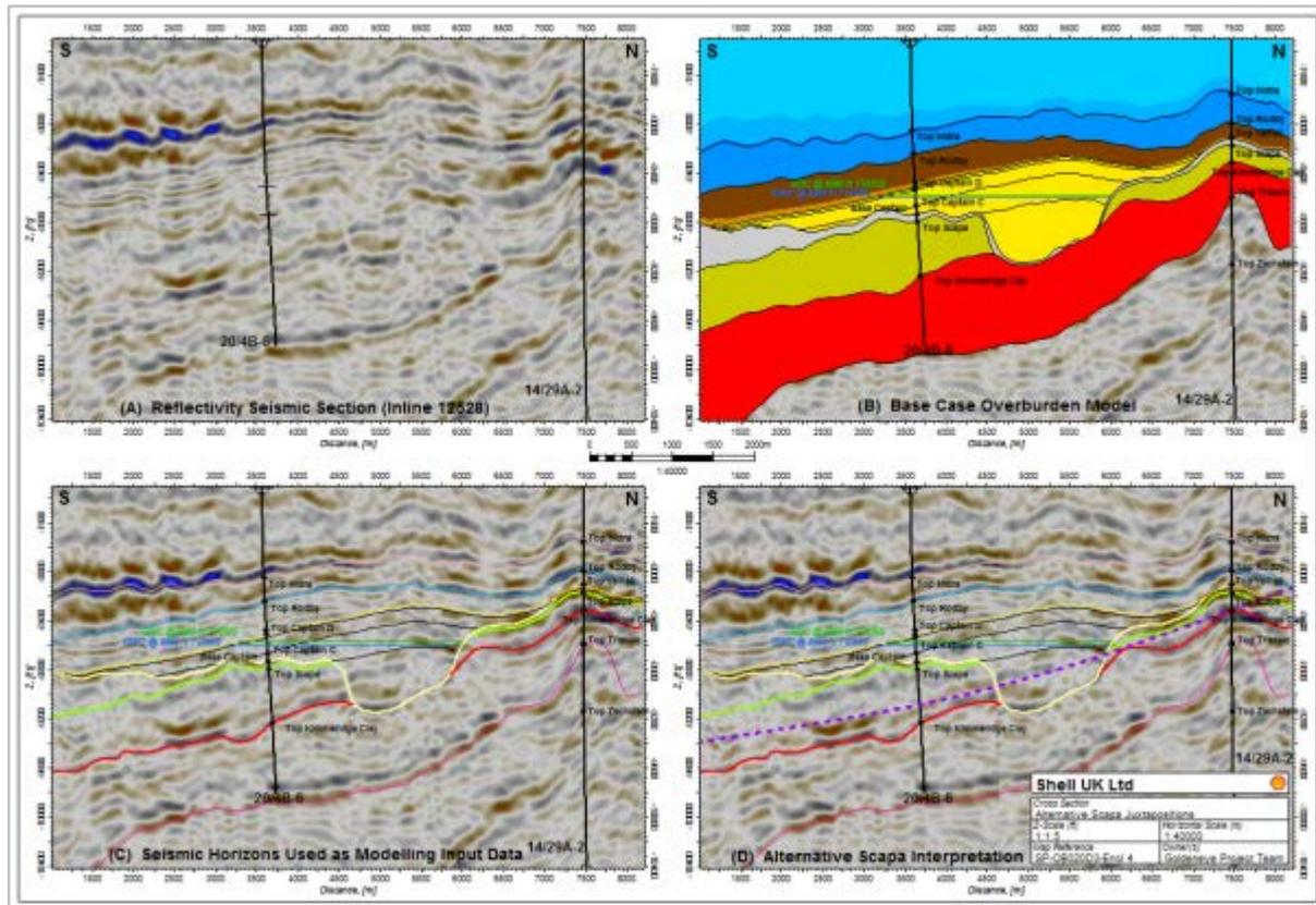
**Figure 9-8 Potential juxtapositions between Captain Sandstone and Scapa Sandstone Members (north-south section between wells 14/29a-2 and 20/4b-6).**
