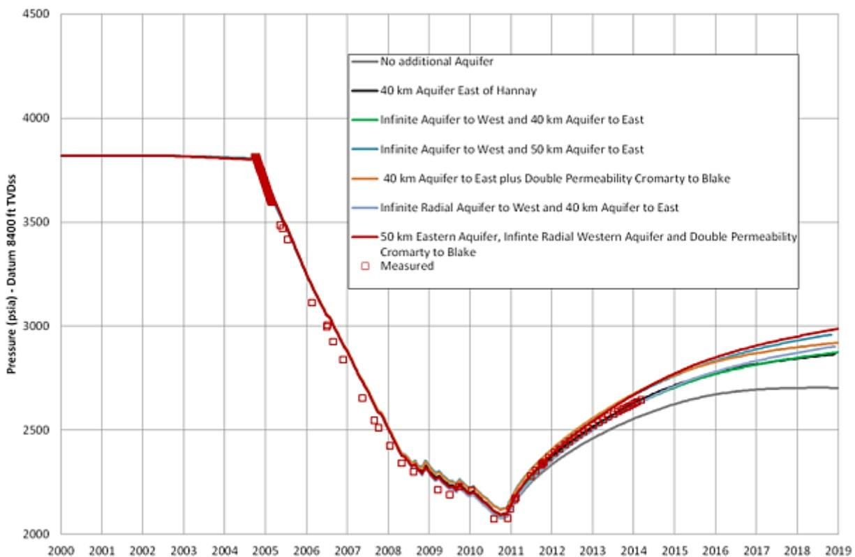
Figure 4-9: Predictions of Goldeneye pressure from field shut-in at end 2010 to 2019
