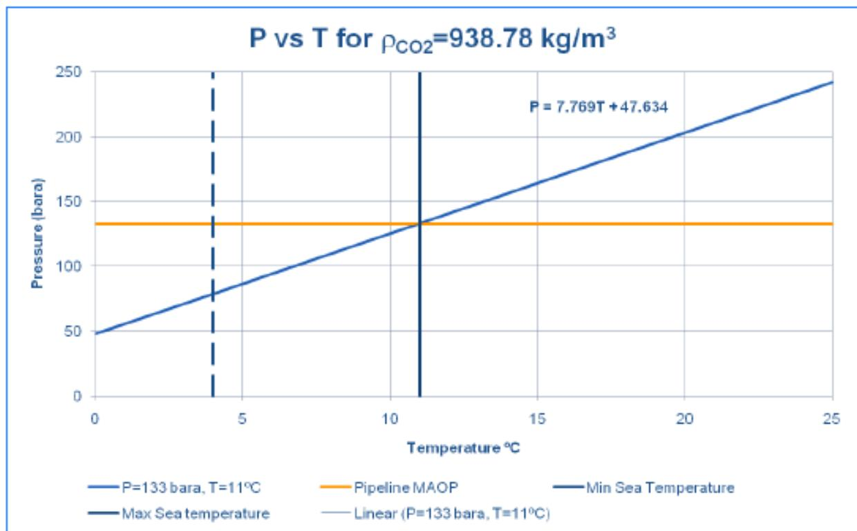
Figure 8-10: Graph showing pressure rise of dense phase CO<sub>2</sub> with temperature.
