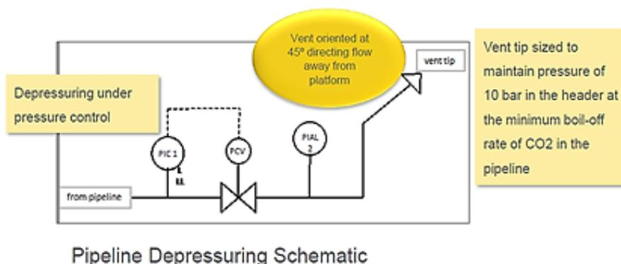
**Figure 8-7: Pipeline depressuring vent schematic.**
