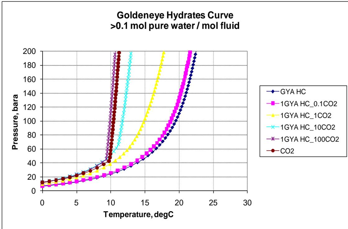
Figure 7-10: Hydrate deposition curve.
