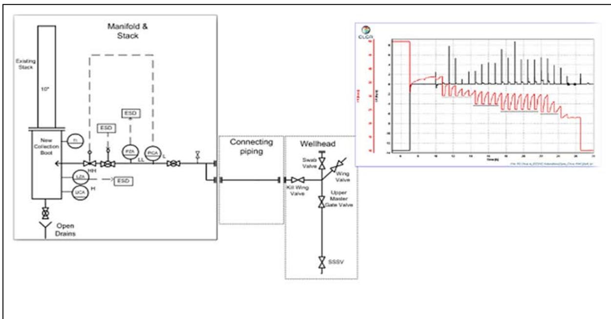
Figure 8-8 Well vent depressuring system schematic.
