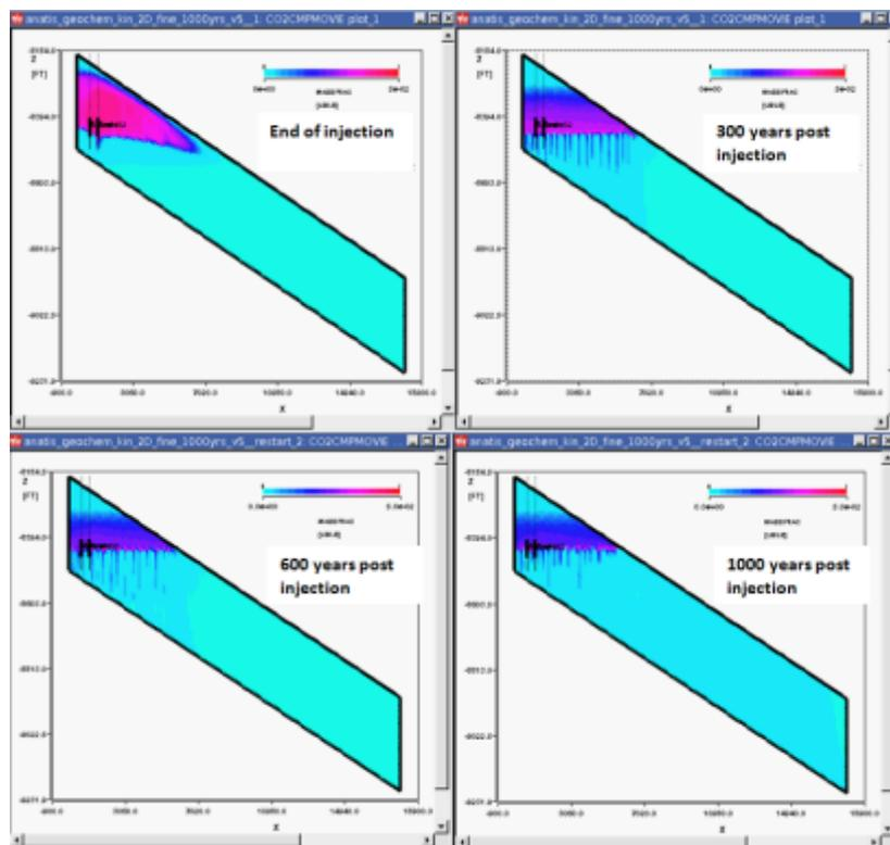
Figure 9-6: Movement of dissolved CO<sub>2</sub> through time (geochemical reaction modelling incorporated). Colour scale runs from 0 to 0.05 (mass fraction).
