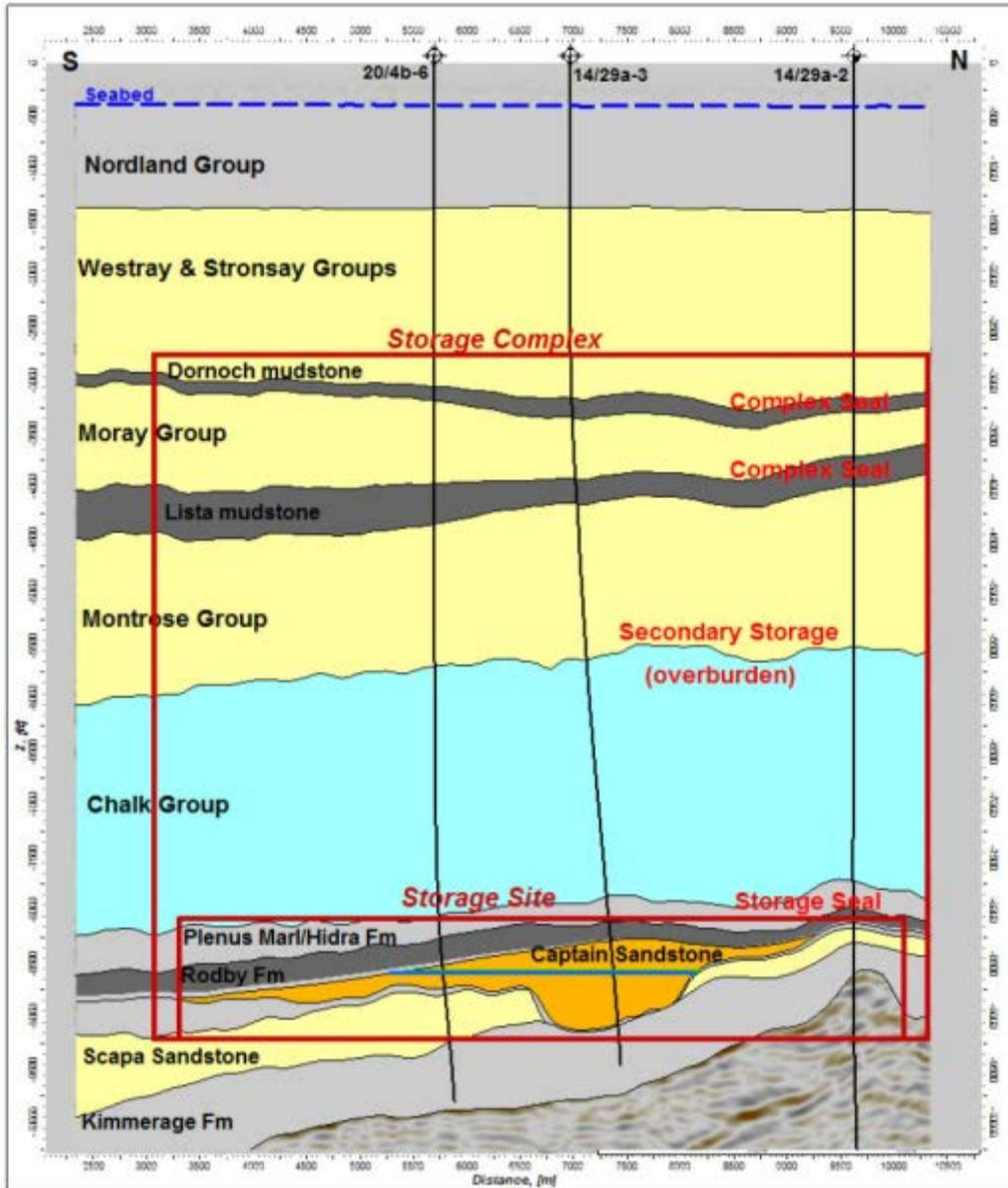
Figure 9-1: Cross section to indicate the vertical (subsurface) extent of the *storage site* and *storage complex*.
