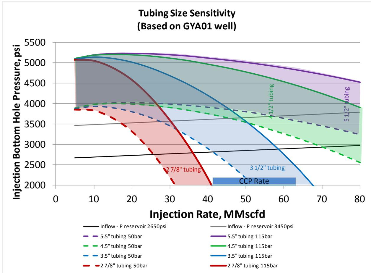
Figure 7-12: Friction dominated concept, sensitivity to tubing sizes
