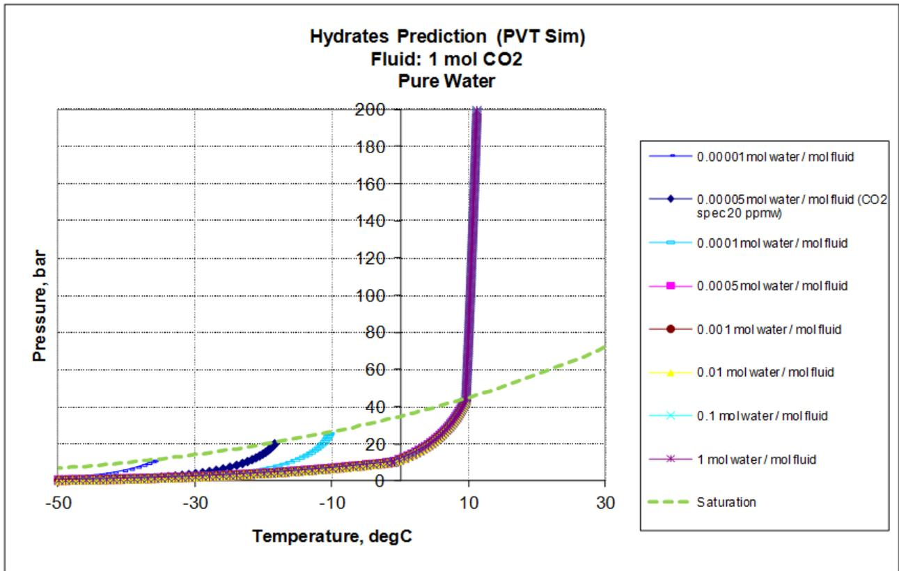
Figure 7-11: Hydrate deposition curve for CO<sub>2</sub> at different water concentrations
