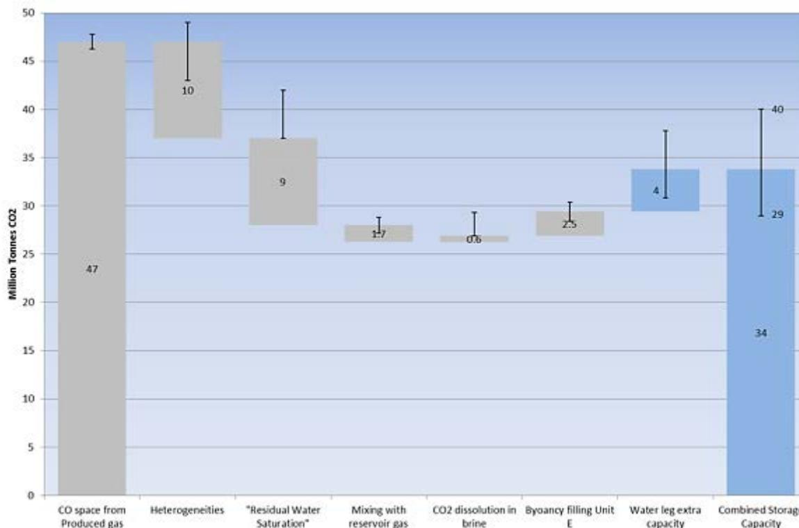
Figure 6-4: Post injection effective storage capacity of Goldeneye (bars 6 and 7 are derived from simulation of 20 Mt injection).
