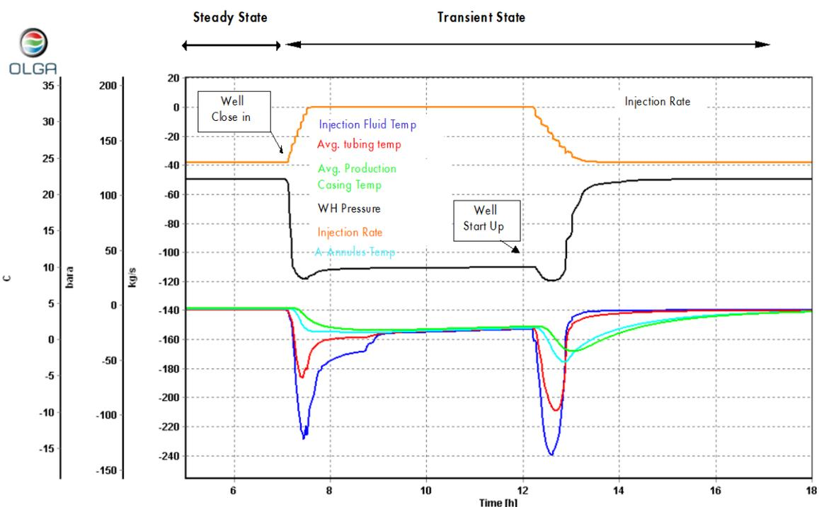
Figure 7-6: Recommended operations case. 4°C IWHT (2500psi P reservoir).
