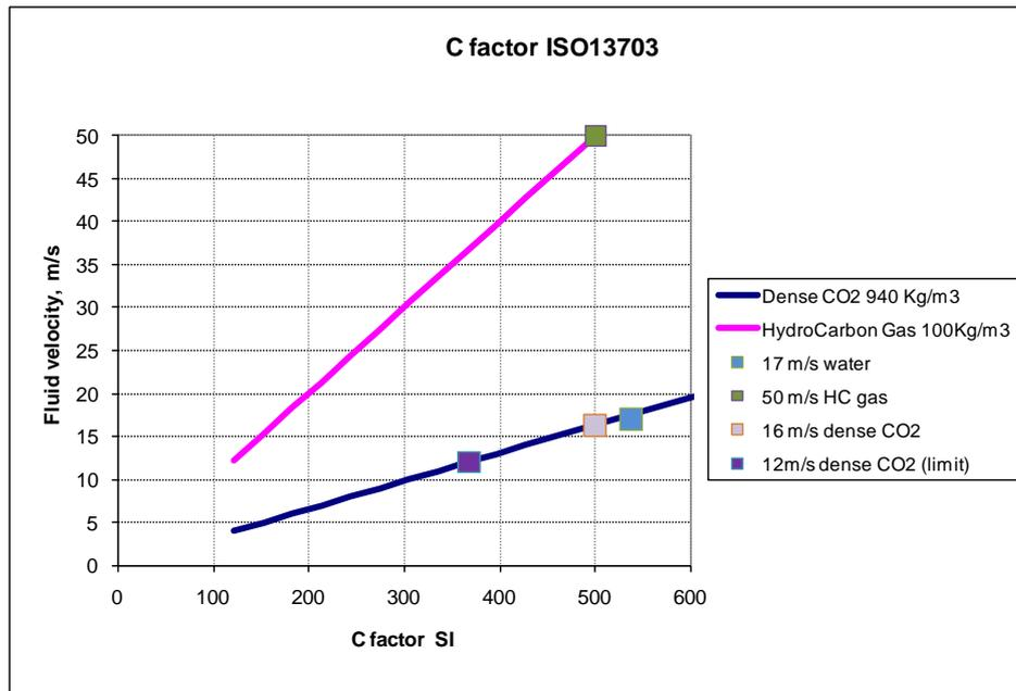
Figure 5-1: C factor comparison (from ISO13703) for CO<sub>2</sub> and hydrocarbon gas.
