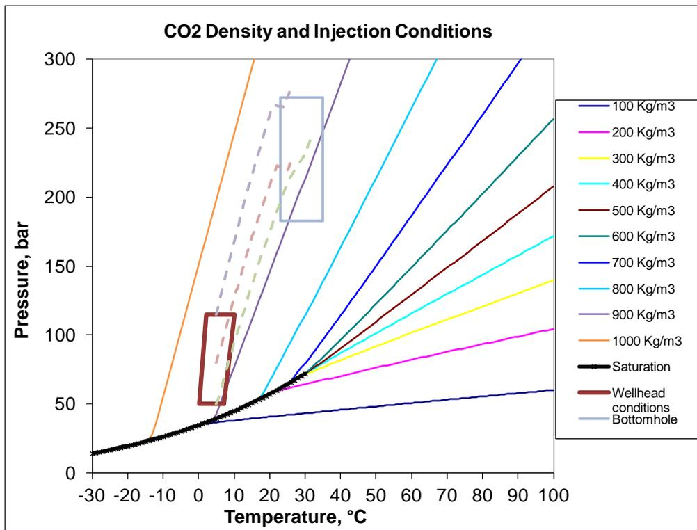
Figure 7-5: Pressure and Temperature prediction with respect to CO<sub>2</sub> phase envelope and density
