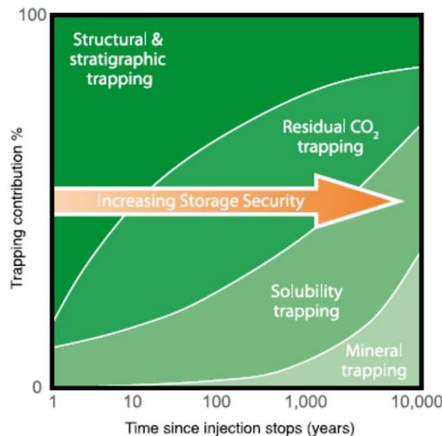
Figure 6-2: Storage security depends on a combination of different trapping mechanism<sup>3</sup>.
