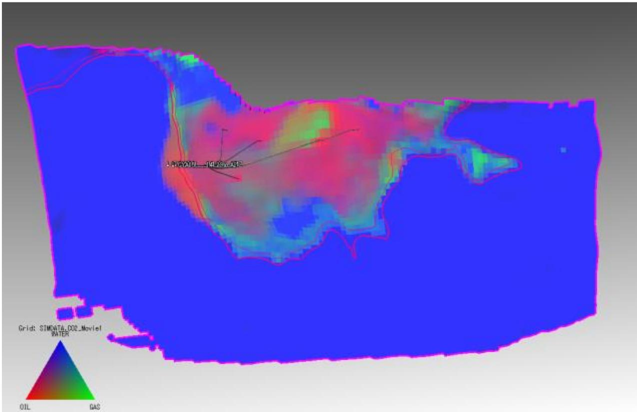
**Figure 9-4: FFM3.1: Extent of CO<sub>2</sub> plume at top Captain D, at end of injection (2029) showing the Dietz tongue on the western flank of the field.**
