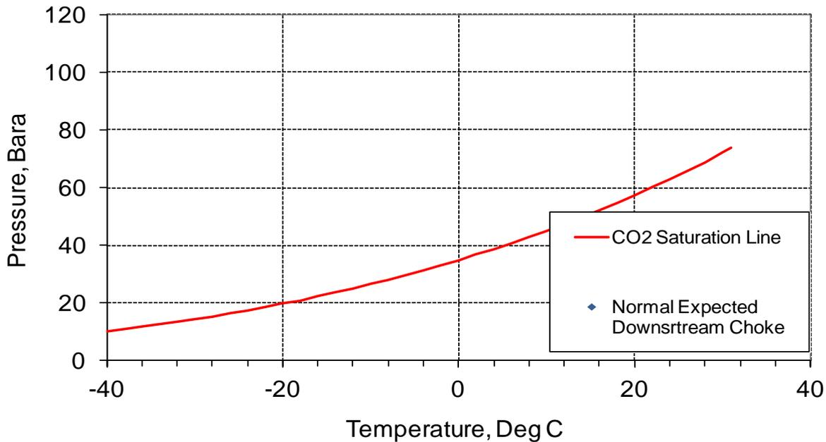
**Figure 7-1: Expected CO<sub>2</sub> choke performance.**
