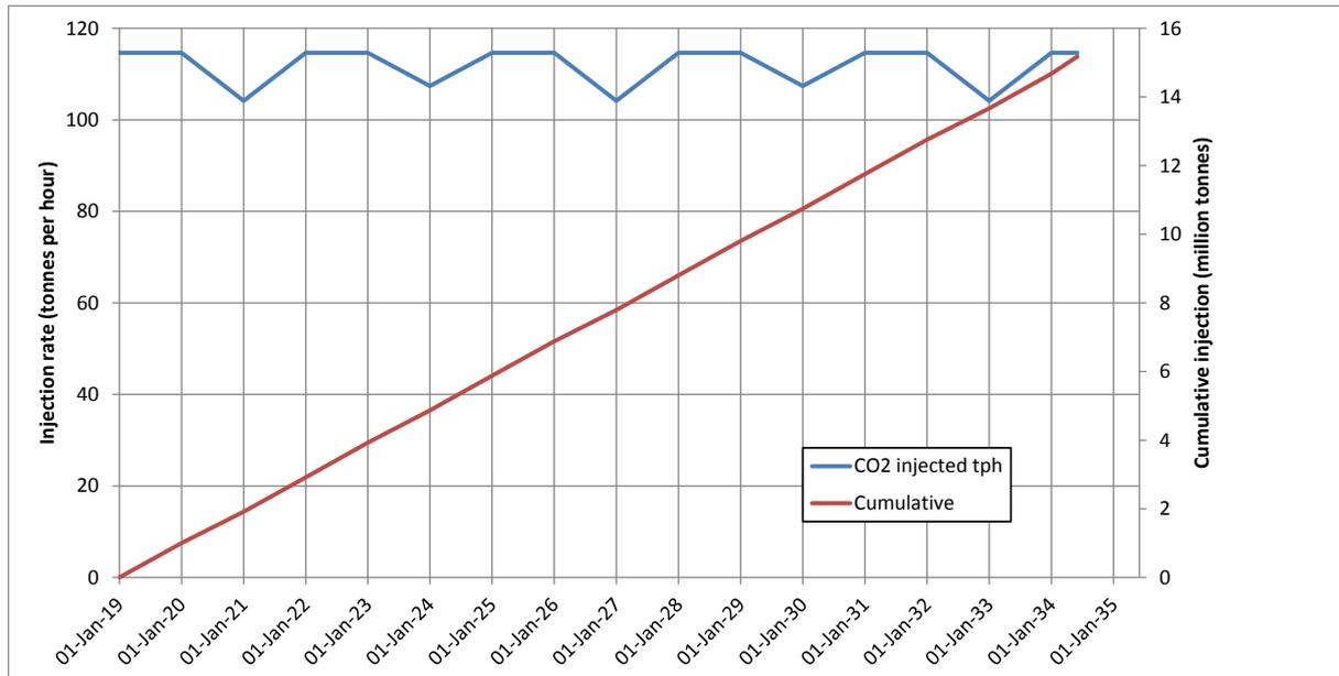
Figure 3-1: Indicative CO<sub>2</sub> injection profile.
