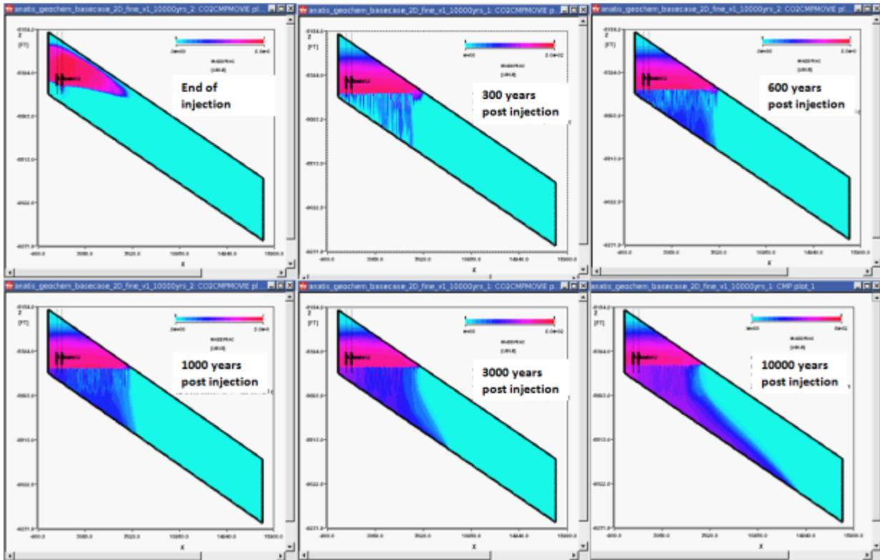
Figure 9-5: Movement of dissolved CO<sub>2</sub> through time (no geochemical reaction modelling). Colour scale runs from 0 to 0.05 (mass fraction).
