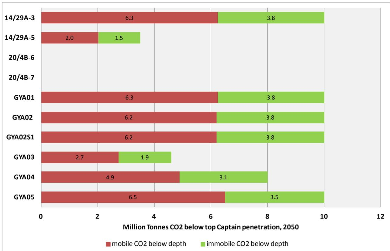
Figure 9-11: CO<sub>2</sub> below the top Captain Sandstone Member penetrations of wells within Goldeneye at year 2050. For 10Mt injection.
