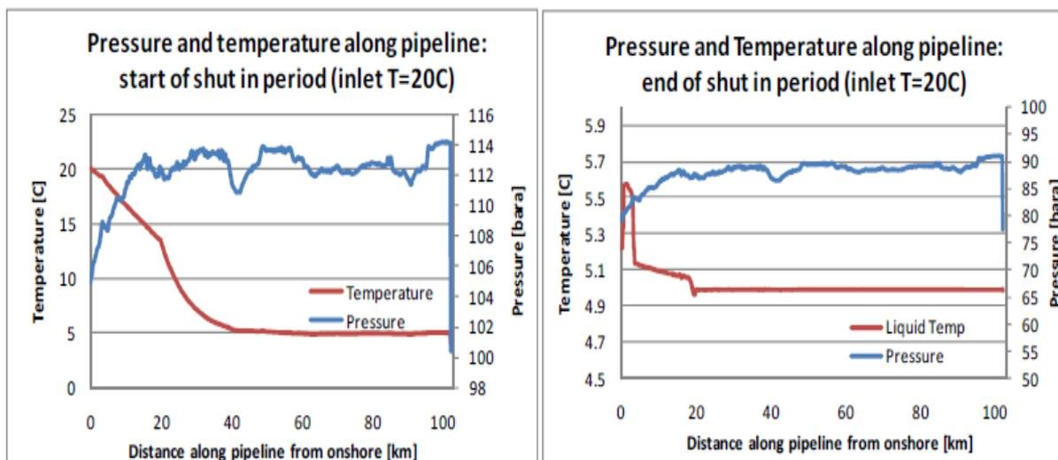
Figure 8-11: Pipeline pressure profile after shut in.
