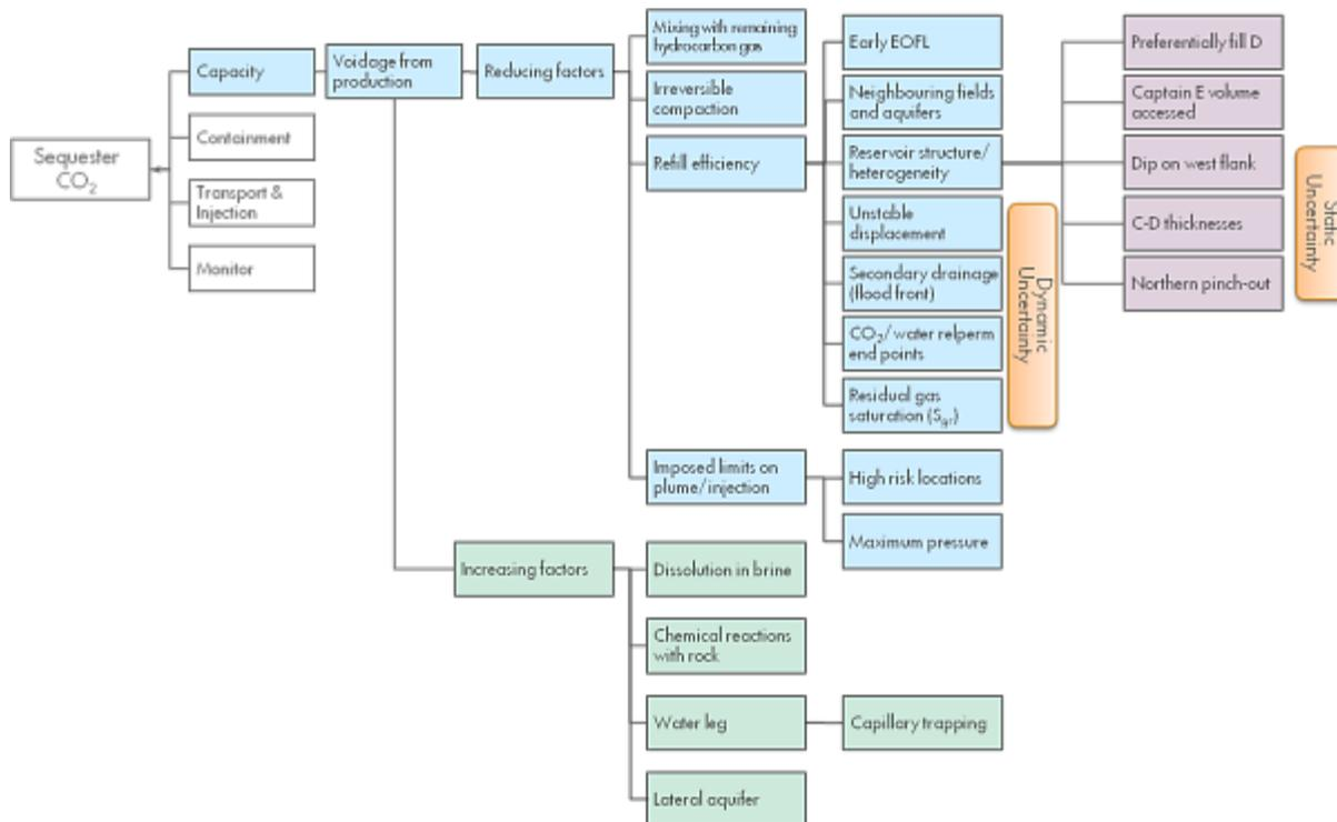
Figure 6-1: Factors impacting CO<sub>2</sub> Storage Capacity.
