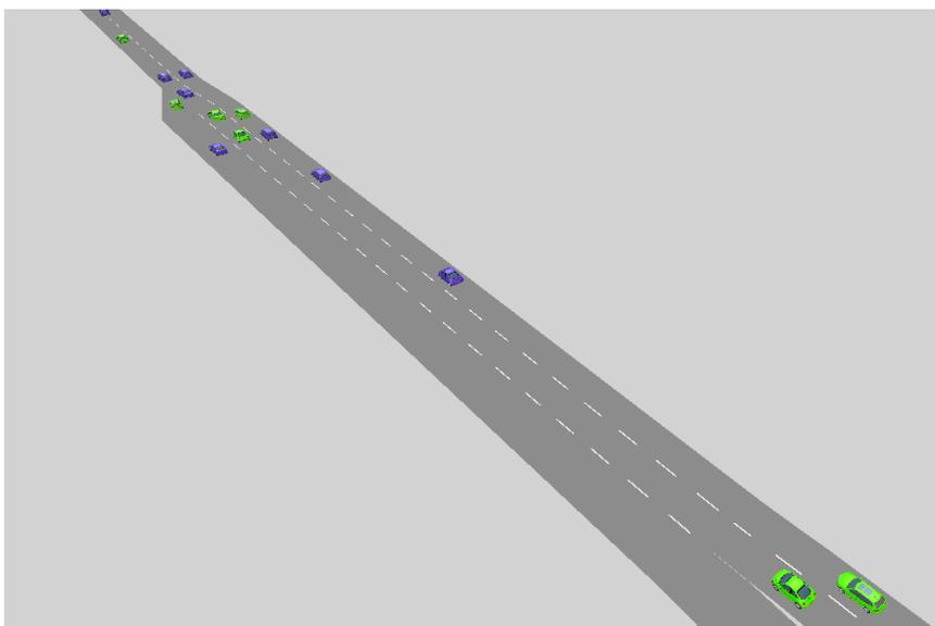
This situation is a typical one on the UK strategic road network, with traffic from another stream joining a multi-lane link. Vehicles on the main carriageway follow other vehicles and may also overtake to attain their desired speed. Vehicles joining the main carriageway at the merge section must identify suitable and safe gaps. The model therefore looks at a range of different behaviours<sup>16</sup>.
