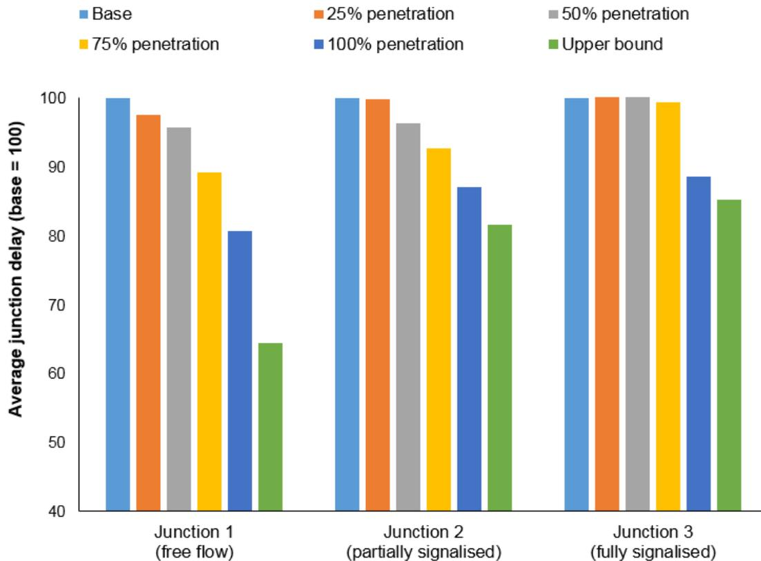
The most significant improvements are seen at the free-flow interchange, with a reduction in delay of as much as 35%. This is likely the situation where the improvements offered by assertive CAVs – high-speed, high-density traffic – can be best realised.
