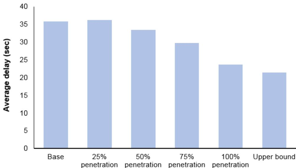
However, with a low penetration of CAVs, some of which will adopt cautious behaviour, total delay can be seen to marginally worsen. Whilst not a large difference, the major conclusion is that a low penetration of low capability CAVs may not result in an improvement to network performance.
