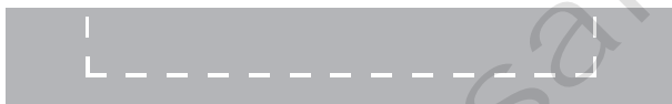
Continuous parking bay adjacent to the kerb (words may be added outside the bay to describe the type of parking)
