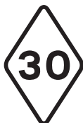
Speed limit sign for tram drivers shown in kilometres per hour. All diamond-shaped signs are for tram drivers only
