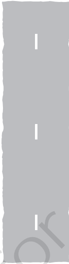
Lane line separating traffic travelling in the same direction (single or dual carriageway road)
