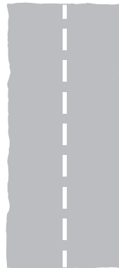
Edge of main carriageway at a junction or at an exit from a private drive. Used in conjunction with 'give way' markings on the side road
