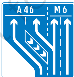
A sign mounted at the side of the motorway shows the arrangement of traffic lanes
