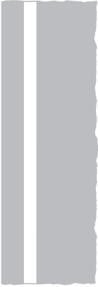
Edge of carriageway, other than at junctions, exits from private drives and lay-bys. Used on the left-hand side of the road and alongside the central reservation of dual carriageway roads
