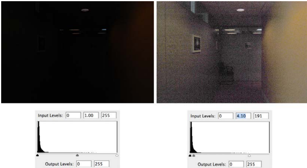
Figure 2 - The image on the right has been brightened using a level adjustment. The histograms show the parameters of the applied level adjustment. Note that although the enhancement has revealed additional detail in the image it has also revealed artefacts in the form of grainy sensor noise.
