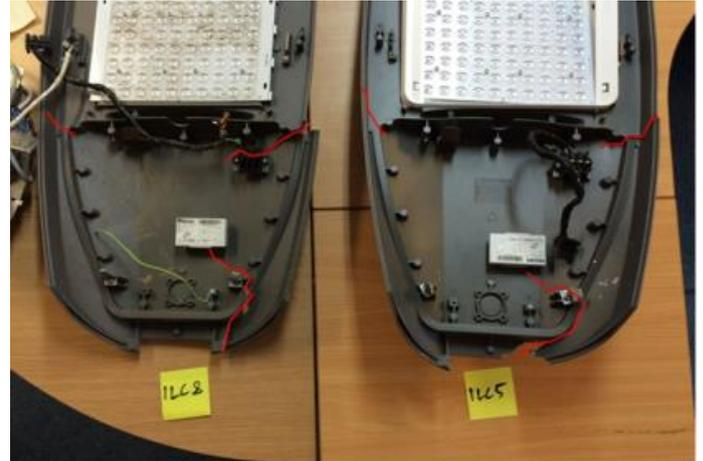
Photo 1: Underside of canopies marked in red to highlight possible material failure
