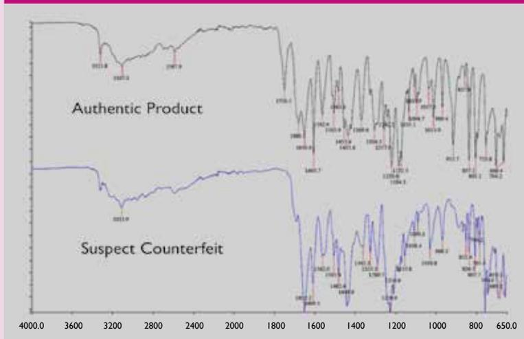
**Figure 3: FT-IR comparison shows that the suspect powder contains paracetamol and caffeine, but no aspirin**
