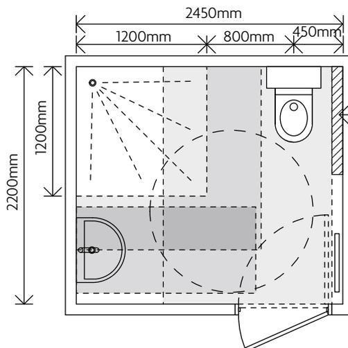
1000 x 1000 x 100mm zone kept clear to enable fitting of rails.
