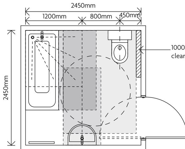
1000 x 1000 x 100mm zone kept clear to enable fitting of rails.
