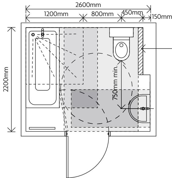
1000 x 1000 x 100mm zone kept clear to enable fitting of rails.
