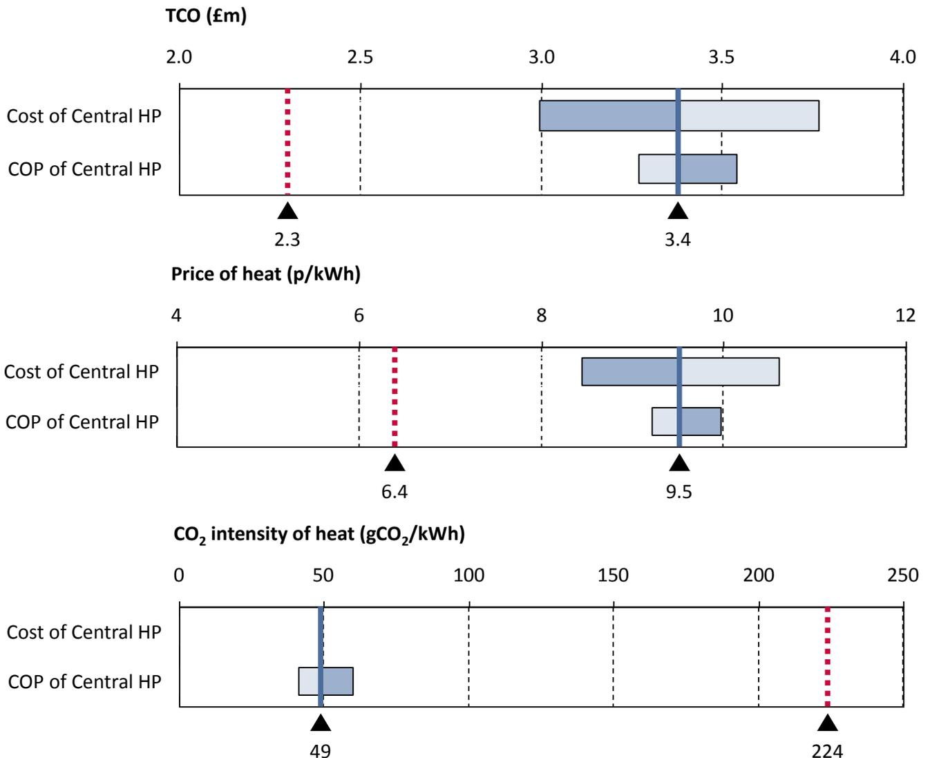
**Sensitivity analysis: Space heating and hot water emitter temperatures**
