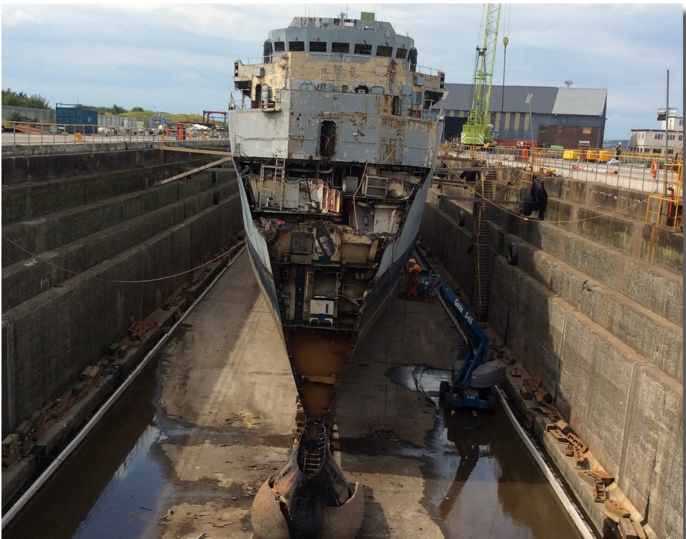
June 2014 Photograph showing the vessel in the dry dock. The vessel is set on blocks with stability bracing and shoring. This bracing and shoring was planned and controlled by the Ballast Water and Stability Management Plans as part of the SRFP. In the foreground is the Sonar Array Dome that required a special plate to split it apart and allow the vessel to be placed on the blocks safely and securely.
