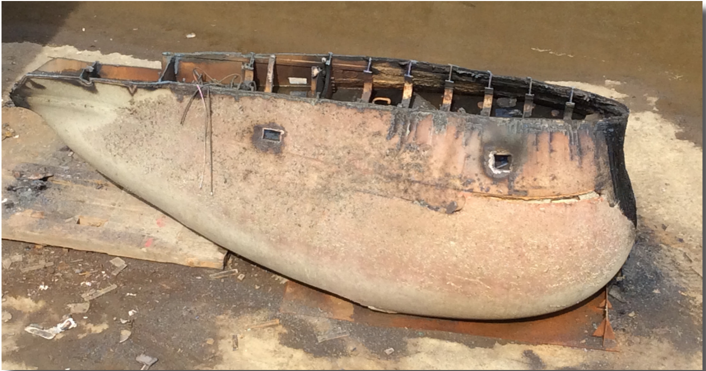
Recycling of the Sonar Dome July 2014. The Sonar Array was removed from inside the dome in one piece. It weighed 15 tonnes and consisted of 64 transducers that yielded over 7.8 tonnes of non-ferrous metal.
