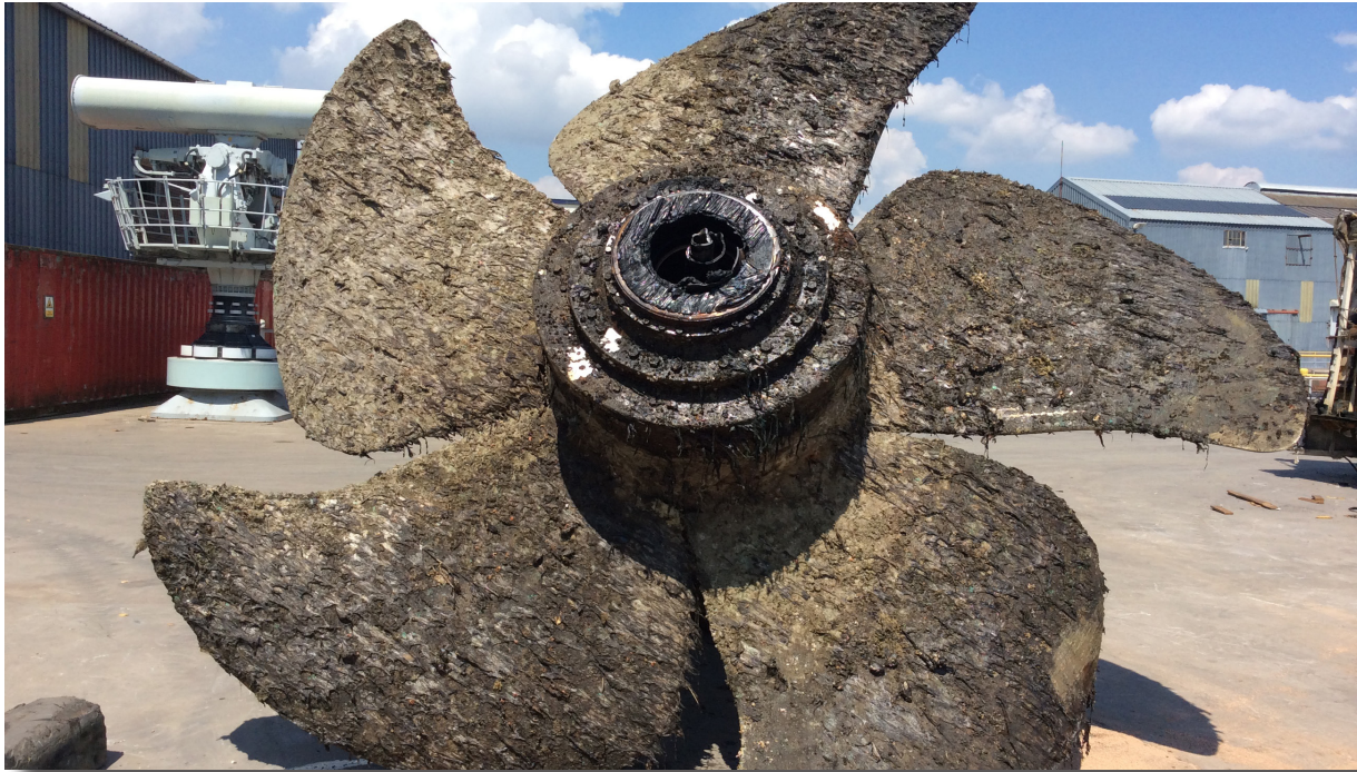
23 June 2014. The propeller once removed was completely stripped down to reveal all of the component parts. Each petal weighed approximately 800kg
