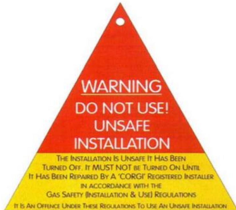
WSG2 — Unsafe Installation Warning Label
