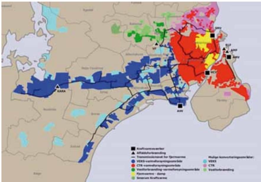
The main part of the network is driven by 10 CHP plants with the total capacity of around 2,000 MW heat. The rest of the heat demand is supplied by a number of heat-only boilers for peak load production. Additionally, some heat is supplied from a geothermal demonstration plant established in 2005, and surplus heat is also exploited from a large waste water
