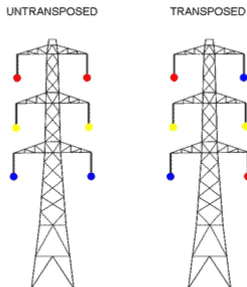
For the normal situation where the currents flow in the same direction in both circuits, the optimum phasing – the phasing that produces the lowest resultant field to the sides of the line - is transposed.
